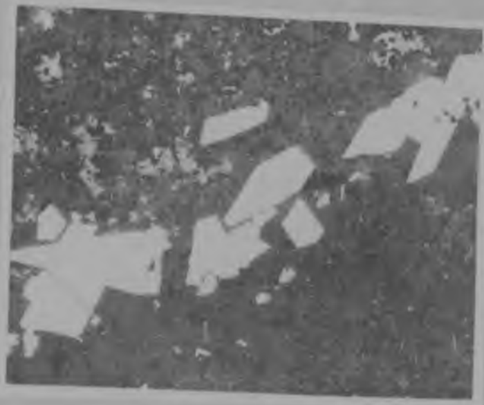
Amphibole in rock. Some amphibole crystals in matrix. Also some small, dark, rounded crystals. Polarized section. Plane polarized \times 50\times .
