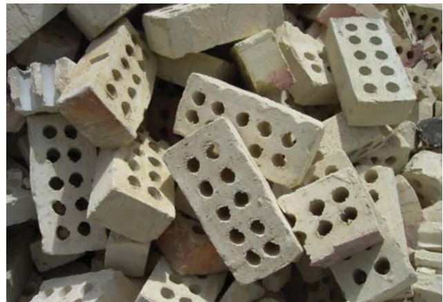
Fig 2.3: Kharuffa, S., 2007. [Photograph] Perforated bricks. Break when wall is demolished. Cannot be reused.
