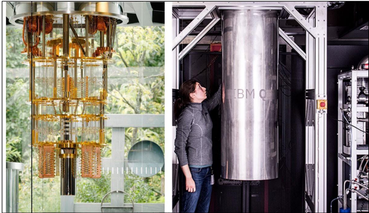
Figure 6.1: (Left) A look inside the 50-qubit quantum computer at IBM. (Right) The enclosure of the quantum computer. [IBM]
