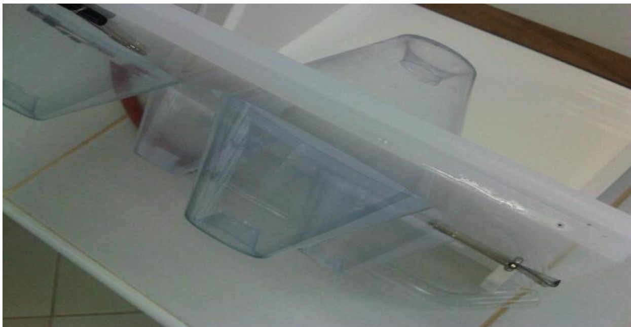
Fig. 2.7 Double cone method of LLIN testing "photo: Pierre Guillet, WHO".
