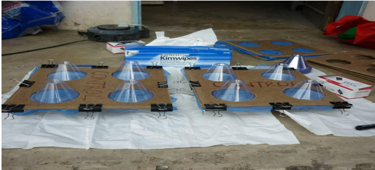
Fig. 2.6 Double cone method of LLIN testing
