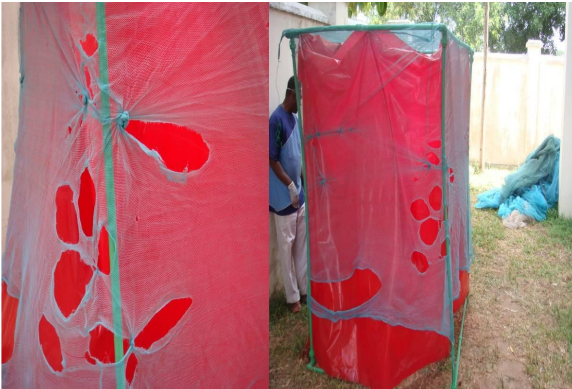
Fig. 3.3 Damaged LLINs being examined on a plastic frame showing distribution of large holes (>5cm) and knots as a method of net repair.
