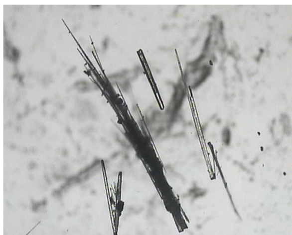
Figure S1. Microscope photographs of (a) block-like crystals of the more stable polymorph I, and (b) the needle-like crystals of the meta-stable polymorph II.
