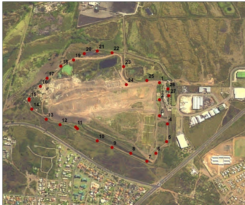
Figure 2.8: Location of subsurface gas probes installed along the boundary of Goudkoppies landfill site (n=27).
