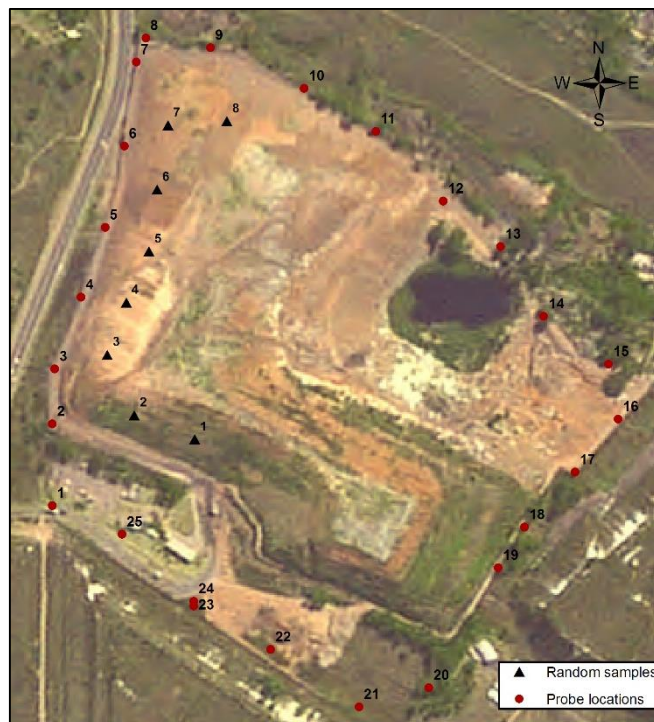
Figure 2.11 Location of flux chambers placed at the surface of the Robinson Deep (top) and Marie Louise (bottom) landfill sites.
