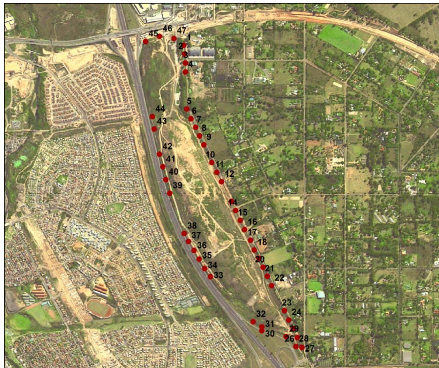
Figure 2.10: Location of subsurface gas probes installed along the boundary of Linbro Park (top), n = 47 and Ennerdale (bottom), n = 27 .
