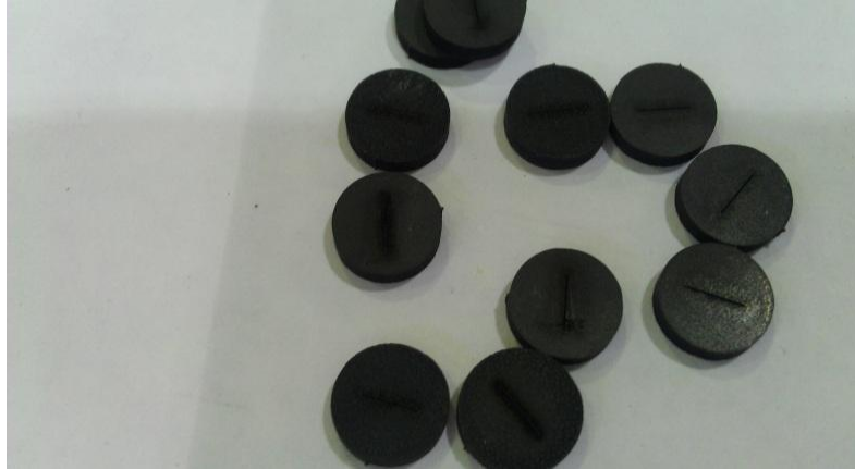
Figure 16: PCD specimen disk prepared for Brazillian Test
