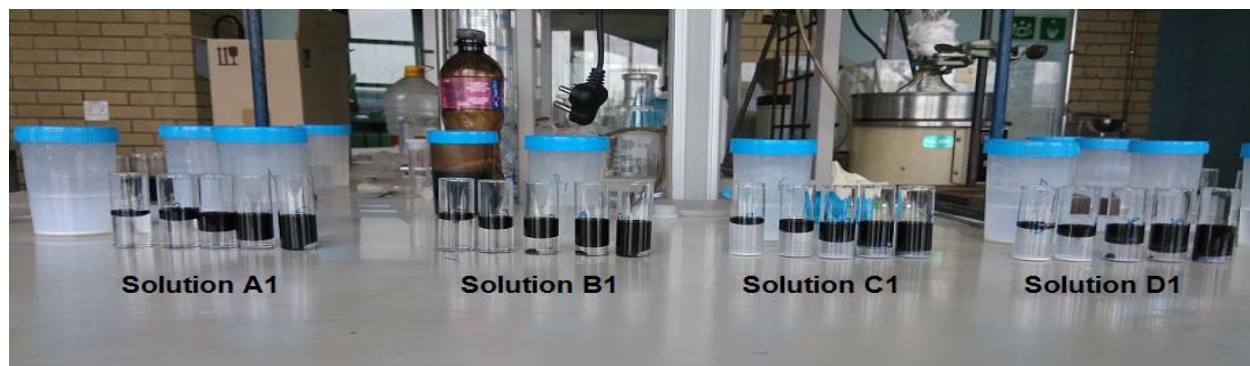
Figure 4.34: the effects on emulsion stability before mixing Experiment 1
