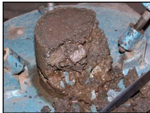
Photo 4.4: Experiment 1: Indication of slurry penetration
