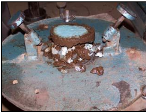
Photo 4.5: Experiment 4: Insufficient slurry penetration
