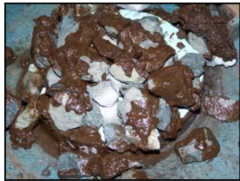
Photo 4.6: Experiment 4: Briquette disintegrated
