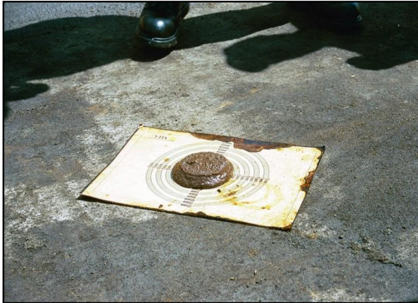
Photo 3.6: Cape Cone Slump test with modified flow plate
