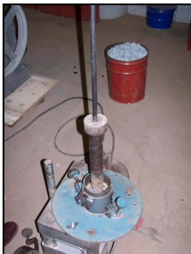
Photo 4.7: Experiment 7: Surcharge weight
