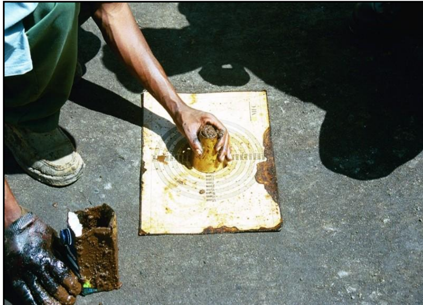
Photo 3.5: Cape Cone Slump test with modified flow plate
