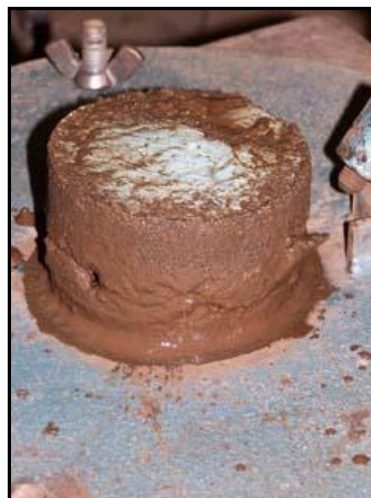
Photo 4.8: Experiment 7: Briquette after early stripping showing excellent slurry penetration
