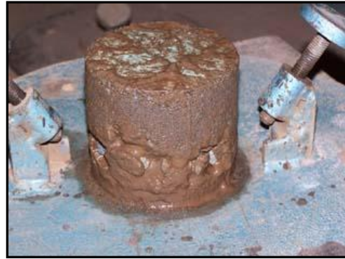
Photo 4.3: Experiment 1: Briquette after early stripping
