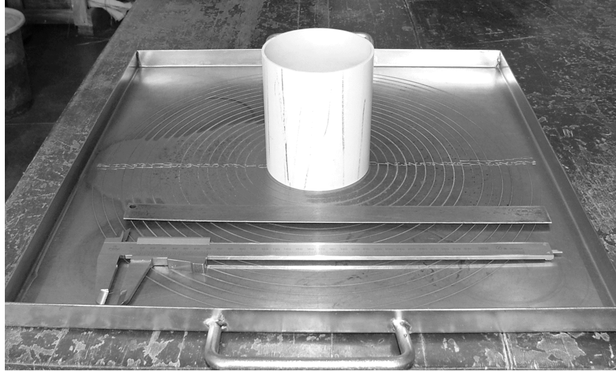
Figure 5.6 : Small slump test equipment
