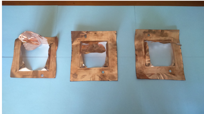
Figure 4.15: Copper diaphragm after test
