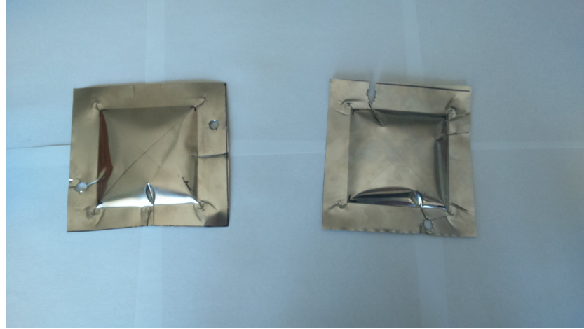
Figure 4.16: Stainless steel diaphragmafter test
