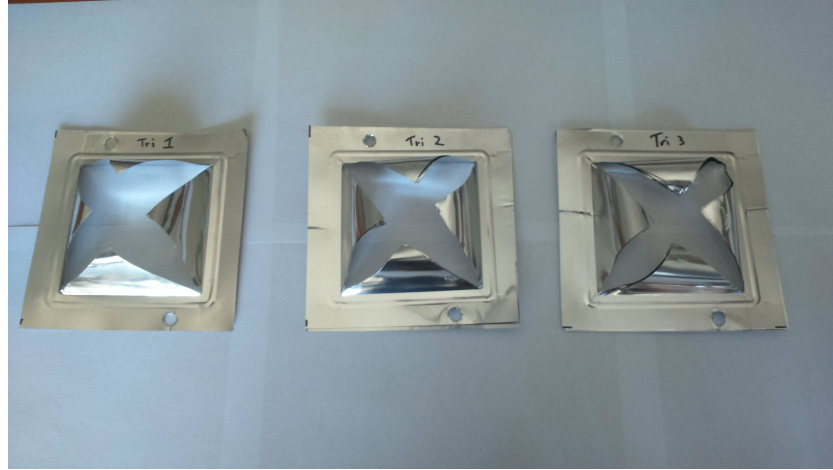
Figure 4.11: Aluminium diaphragms after burst, left: 1 diaphragm used, middle: 2 diaphragms used, right: 3 diaphragms used
