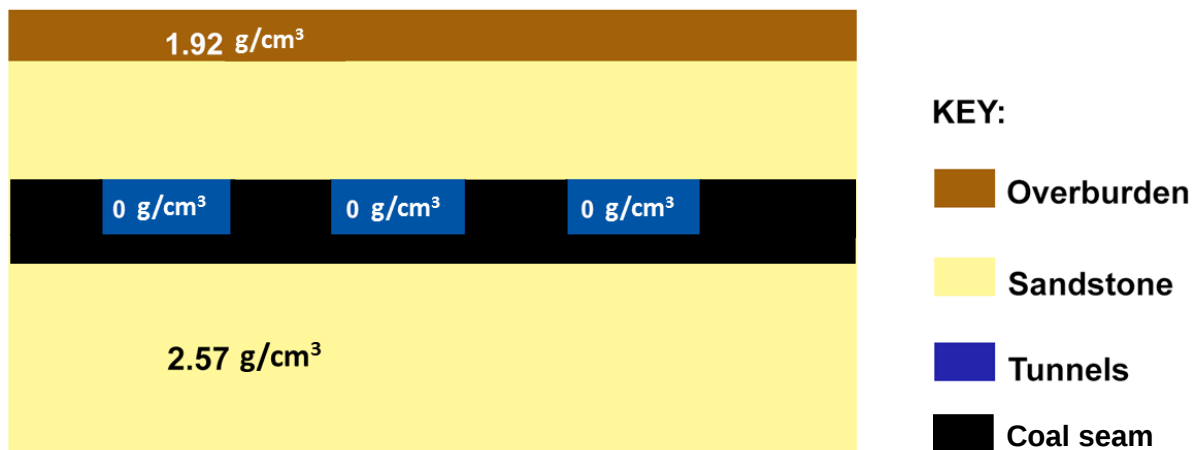
Figure 2.10. A postulated vertical geological section based on observations used to guide 2D forward modelling of microgravity and magnetic methods. The model shows a postulated unrealistic horizontal overburden that was eventually superfluous in the final microgravity models as with gravity, horizontally layered strata only contribute to the background or regional gravity field and bodies must be at least slightly dipping or change in the vertical dimension to produce an anomalous effect, for instance uneven weathering. The tunnels in the model are designated by the blue squares with a strike length of 50 m in both directions and with a density of 0.0 \text{ g/cm}^3 which was taken as the practical density of air. The host rock is the sandstone. The black coal seam is included in the section to show the position of the seam along the tunnels. It must be noted that this is an ideal case, but the pillars are not entirely coal.
