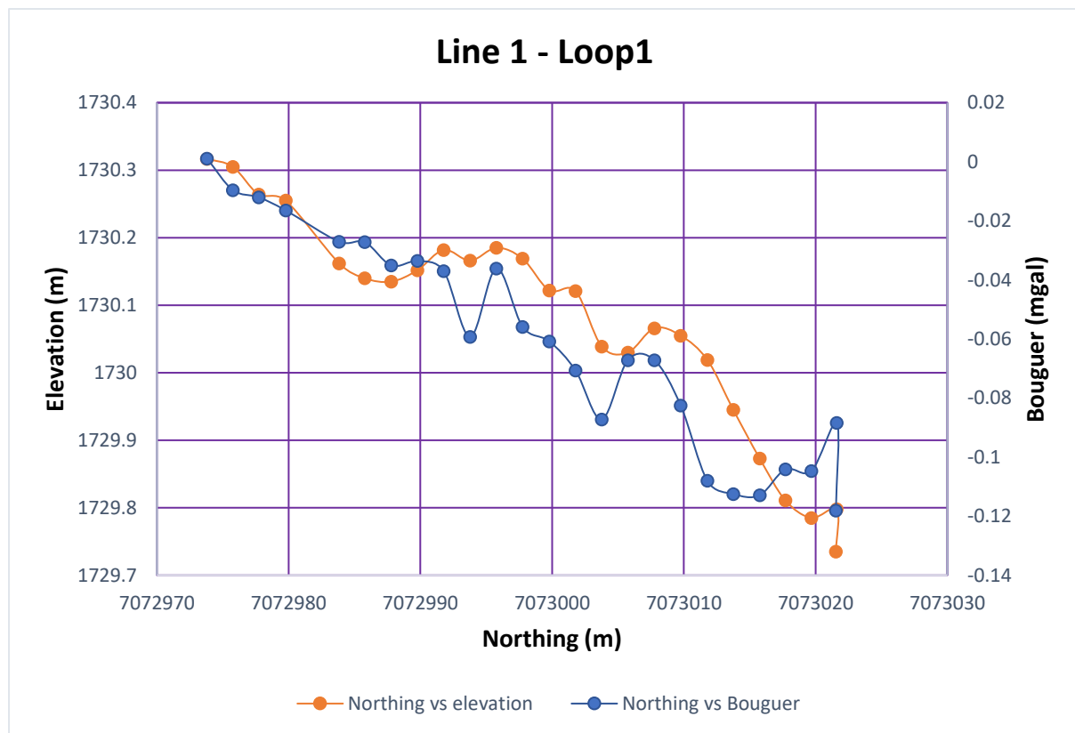
Figure 4.4. A plot of line 1 which is the first loop showing plots of elevation (m) and Bouguer anomaly (mgal) against northing. From the figure, the variation of the amplitude in mgal of the anomalies is \pm 0.03 mgal and no regional trend is removed yet. This loop has 1 internal and 2 external (on loop 2) repeat measurements. Although there is a positive correlation between the elevation data and the BA values, this is considered fortuitous as the variation in BA values is much more than the variation in elevation differences (these have a 0.2 m maximal value).
