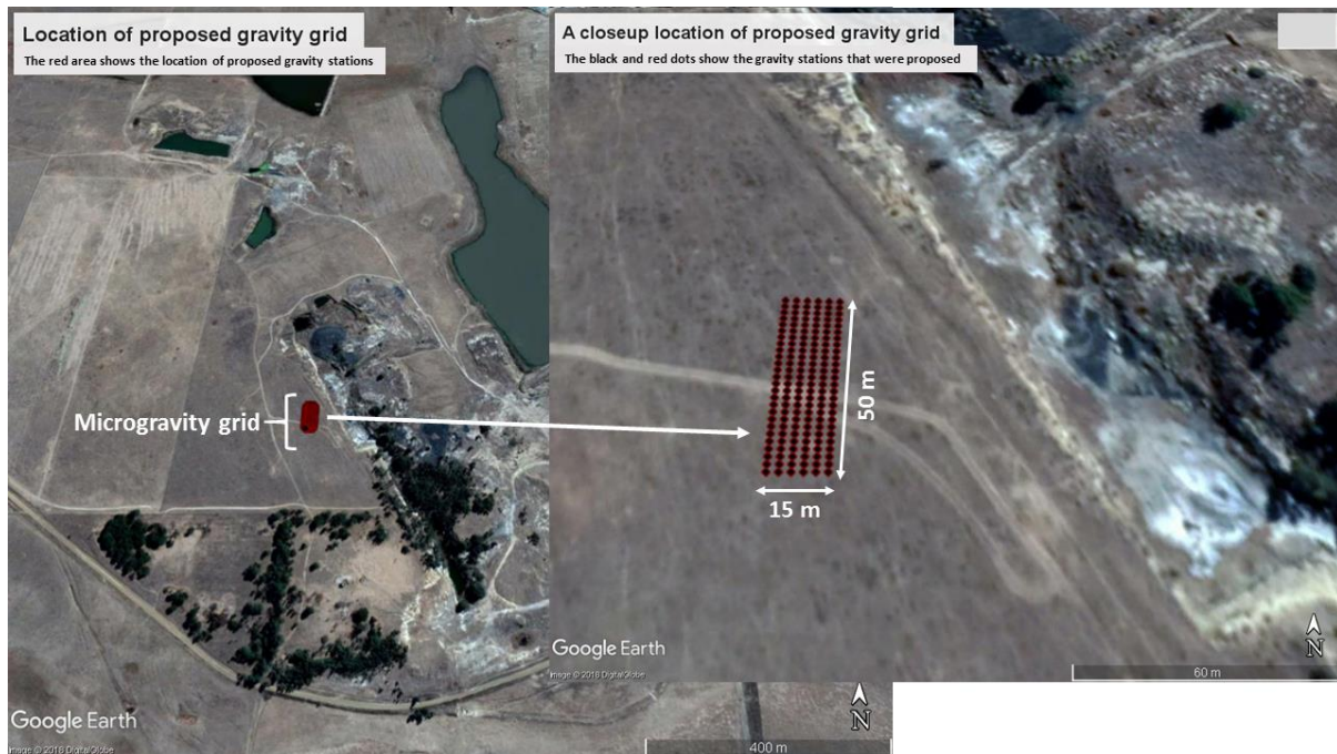
Figure 2.1. Google Earth image showing proposed location of the microgravity grid (in red) plotted on Google Earth (using Global Mapper13). On the right of the grid is the access to the tunnels and the insert image depicts an enlargement of the grid location.
