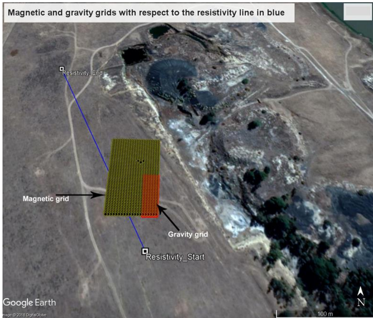
Figure 2.7. A picture showing a planned microgravity (red) and magnetic (yellow) grid patterns (using Global Mapper13) based on the position of the resistivity line (blue).
