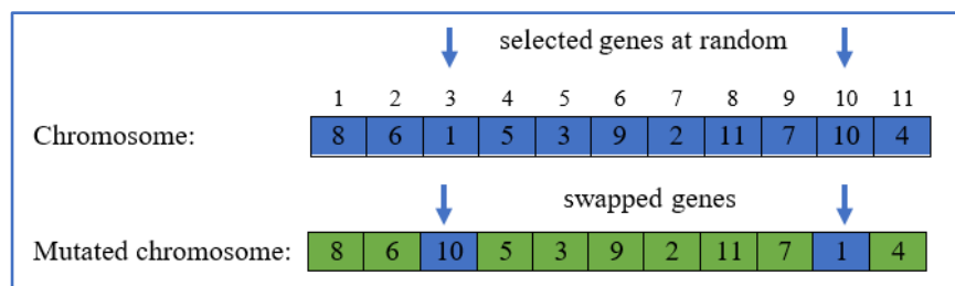
Figure 2.14: Illustration of the swap mutation genetic procedure (Source: adapted from Gen et al. , 2008)
