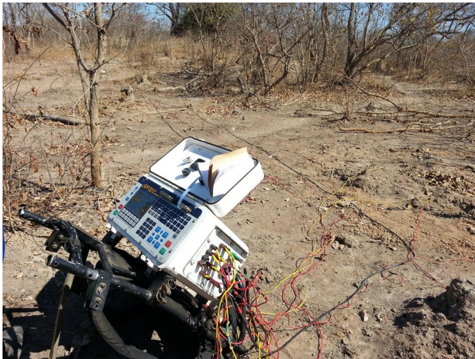
Figure 5.1. Zonge GDP- 32 24 multi-receiver system for acquisition of controlled and natural source geoelectric and EM data.
