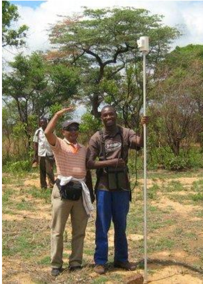
Figure 4.15. G-856 proton precession magnetometer used to take magnetic measurements.
