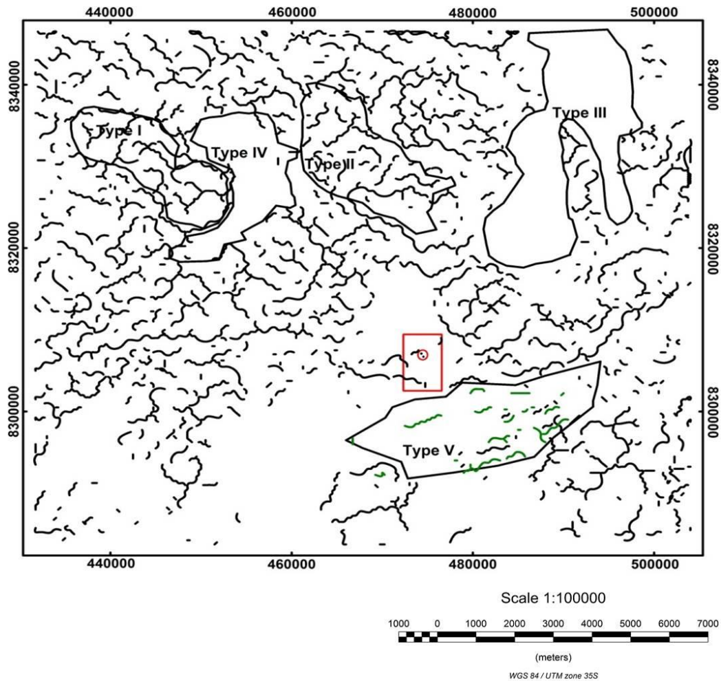
Figure 4.9. Map of the negative magnetic lineaments mapped using phase symmetry algorithm that was developed by (Kovesi, 1997). A smallest filter wavelength of 500 m, and 4 filter scales were used to detect negative magnetic lineaments (black) orientated at all angles and positive magnetic lineaments (green) outlined in Type V anomaly.
