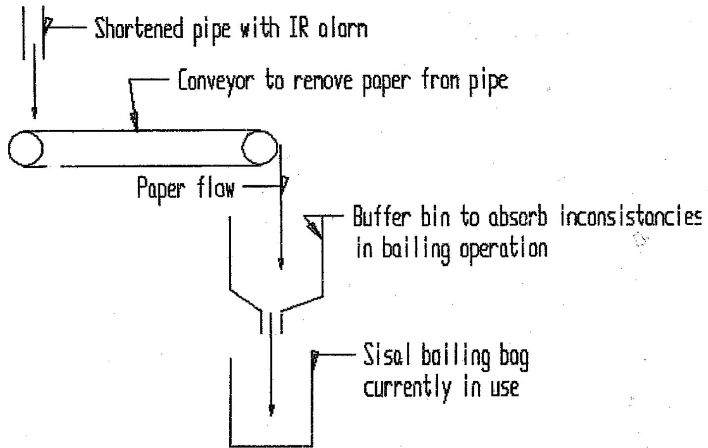
Fig. 9.3 Conveyor belt installed in bailing room to prevent pipe blockages
