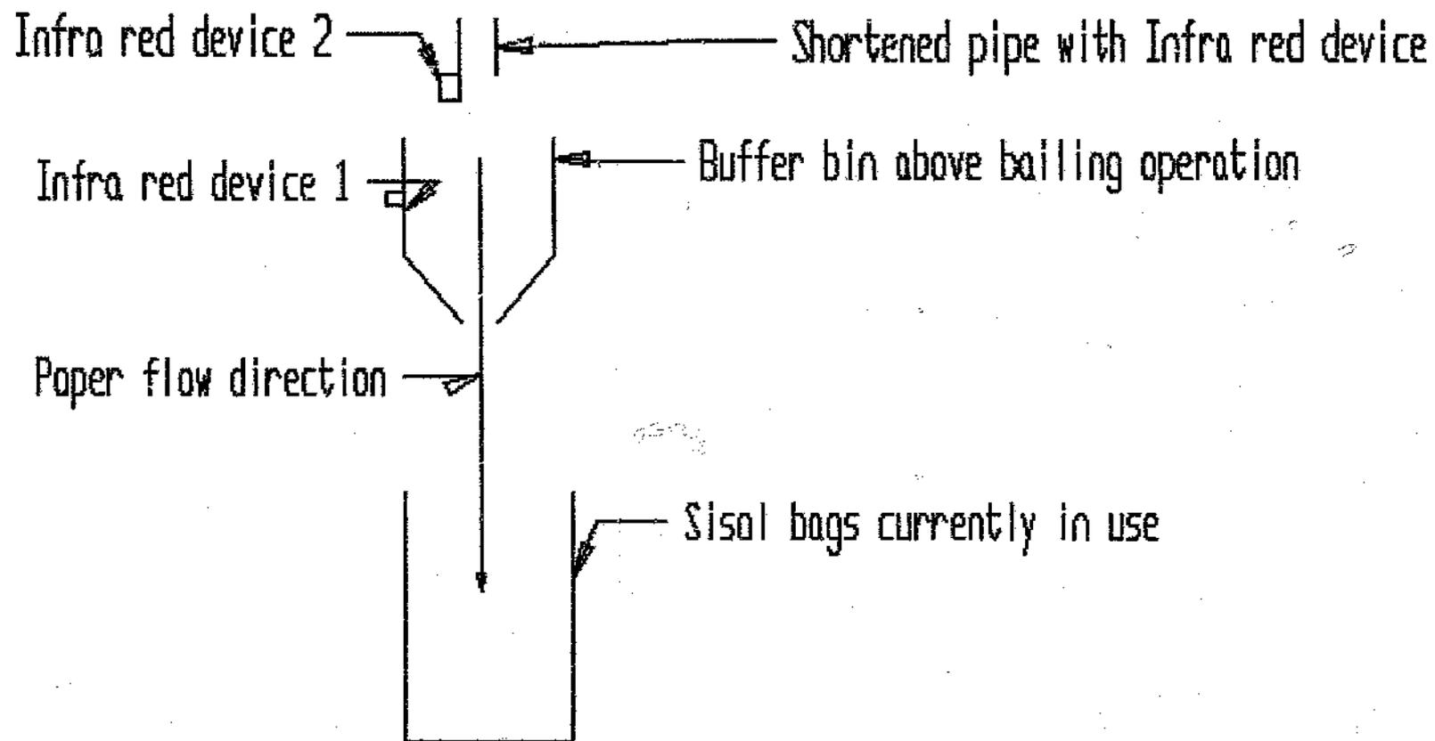
Fig. 9.2 Bailing operation utilizing a buffer bin and alarm systems to signal blockages
