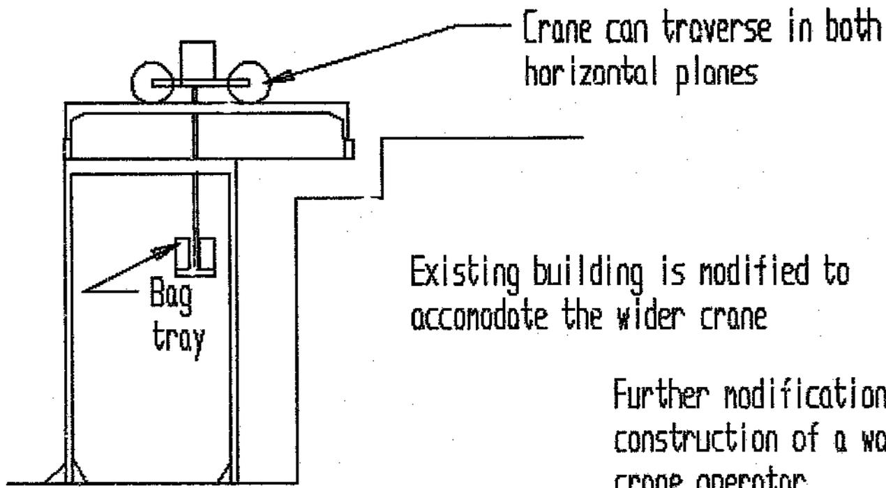
Crane can traverse in both horizontal planes
