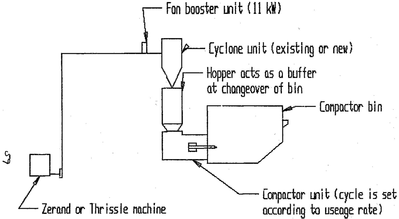
Fig. 9.5 Compactor used on Zerand and Thrissle machines
