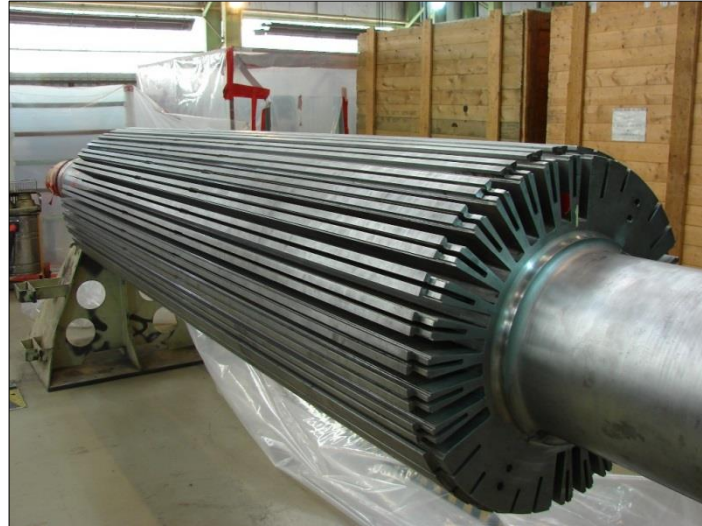
Figure 3.2: Generator rotor body with final machined winding and cooling slots
