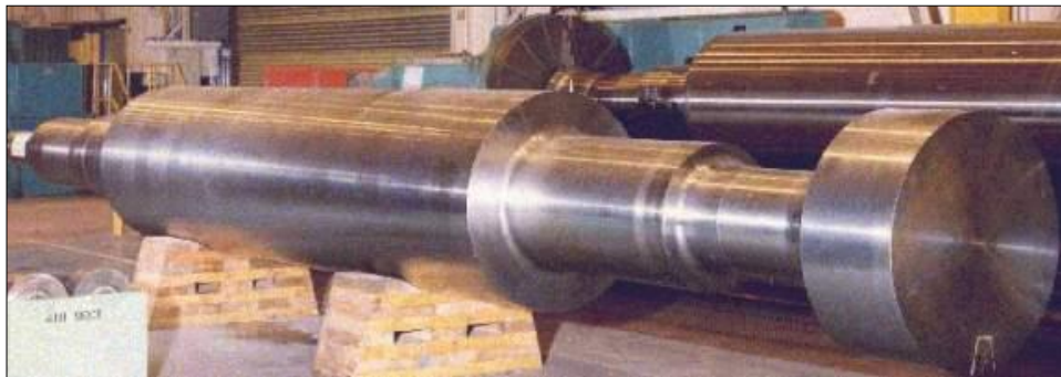
Figure 3.1: Generator rotor rough machined mono-block steel forging
