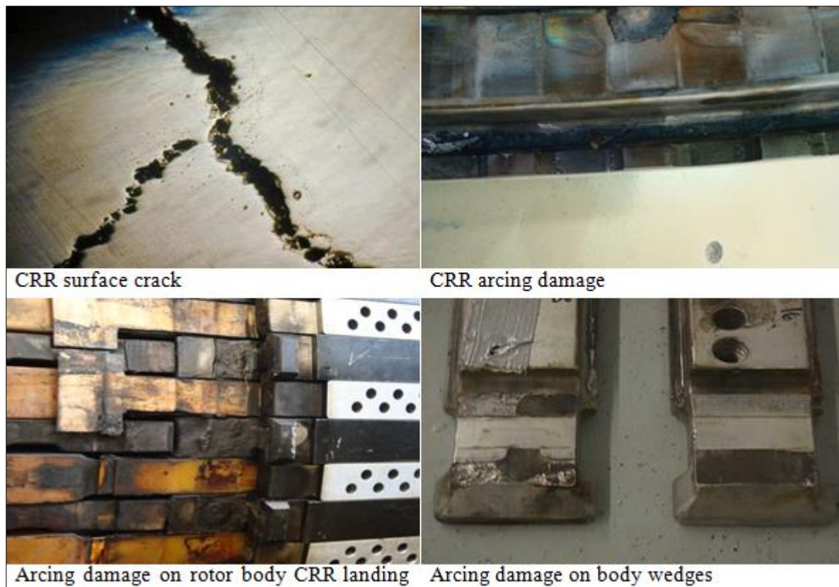
Figure 2.4: Common turbo-generator rotor body failures: cracking, arcing
