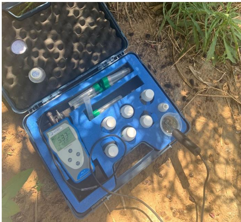
Figure 14: A photo showing pH, temperature, and electrical conductivity testing on one of the sampling sites.
