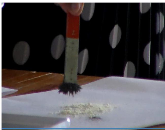
Teacher using magnet to separate iron fillings from sulphur powder.
