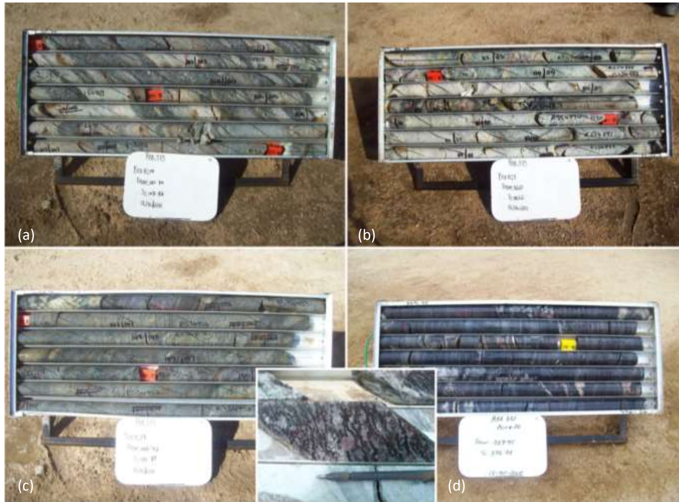
Figure 3.32 Typical Rössing Formation lithologies observed in Zone 1 drill core specimens. (a) The upper units of the Rössing Formation are eroded away in parts of Zone 1; the intercalated diopside gneiss, quartzite and calcsilicates shown from RDD373 at ~100 m depth correlate to the upper marble sequence at the Rössing Mine. (b) The impure upper marble typically contains serpentine - diopside carbonates, quartzites and occasional skarns where intrusives have provided heat \pm fluids. Intercalated gneiss and calcsilicates typify the package. (c) The dominant pelitic unit(s) include a thick ~10 - >100 m thick cordierite gneiss, which is variably metamorphosed and contains conspicuous amounts of hydrothermal sulphide mineralisation. The typical units include chloritic, migmatized cordierite gneiss, banded and augen garnetiferous gneiss and calcsilicates. (d) Lower pelitic units usually are separated by a carbonate unit(s) from the upper cordierite gneiss. These are distinguished by darker colour, significantly less prominent chlorite and a prominent garnet porphyroblasts (e - inset). The examples shown above are from diamond drill holes RDD373 and RDD351.
