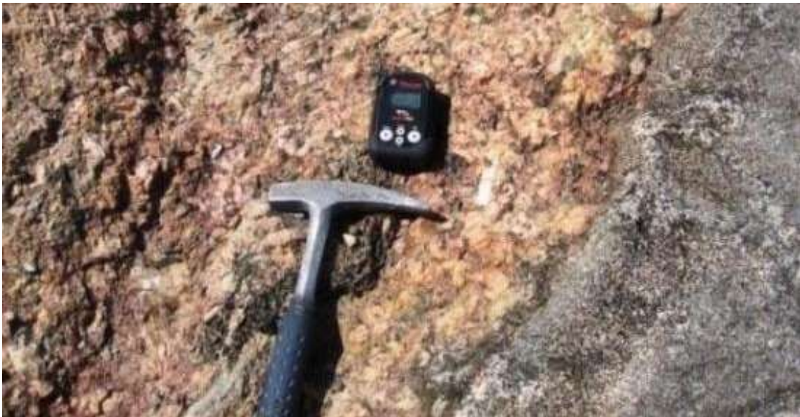
Figure 3.59 Typical mineralised sheeted leucogranite texture at Hildenhof. Mineralised Sheeted leucogranites at Hildenhof are coarse to pegmatitic with highly variable biotite content. The sheets intrude pelitic metasediments, and biotite laths at the margins reflect the orientation of the sediments.
