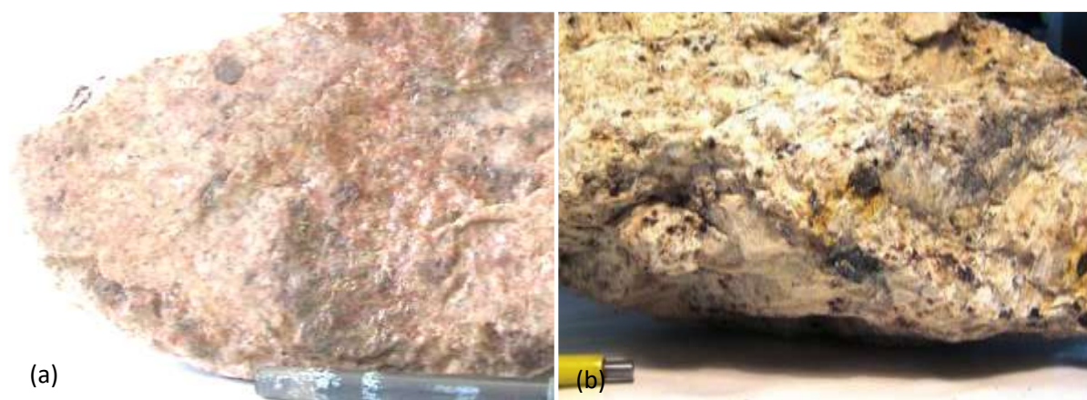
Figure 9.3 Textural varieties of garnetiferous leucogranite. It is not absolutely certain if the two varieties represent the same anatectic melts of the Kuiseb schist described by Ward et al. (2008) but the two types (foliated, left, and pegmatitic, right) have distinctive temporal-, petrographic-, and consistent geochemical contrasts.
