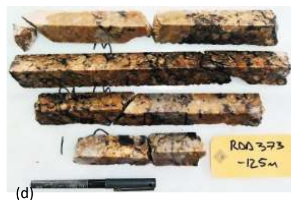
Figure 5.56 The RDD373 124-125 m sample with thin section locality and handheld XRF assay data. The sample is an altered alaskite with prominent biotite content and pervasive fracturing throughout the mineralised interval. High cps readings are localised over biotite clusters. (a) A systematic 10 cm assay scheme with handheld XRF values highlights discrete sites of elevated Nb with corresponding elevated Ti. (b) The sample is situated in an 8-m thick pegmatite-alaskite with prominent coarse-grained biotite. (c) The department study by QEMSCAN reveals 10 wt.% U in betafite combined with brannerite for 16.94 wt.% U in refractories. This sample in particular shows that potential exists for XRF analyses as a means of identifying refractory-bearing targets. (d) Illustration of the distinctive alaskite texture.
