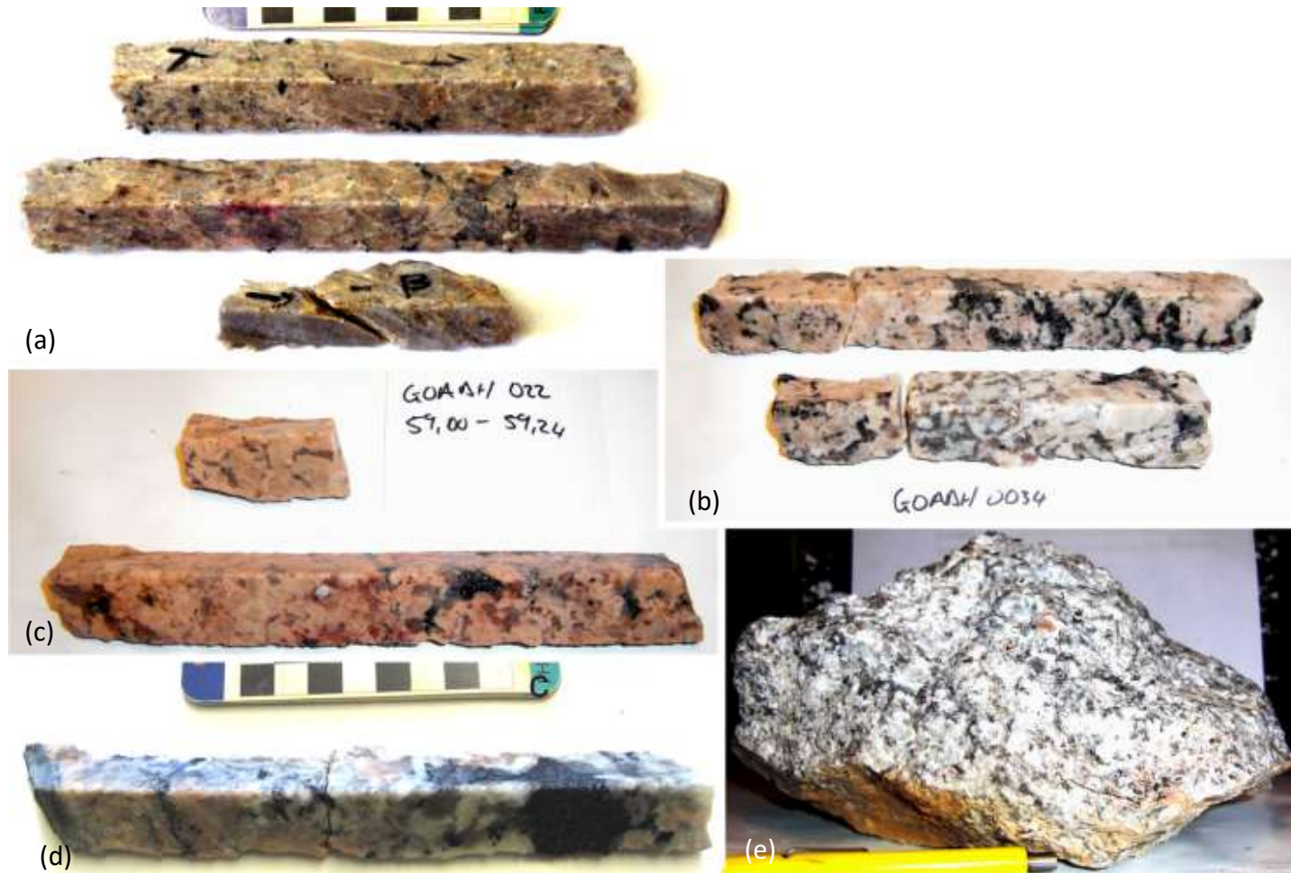
Figure 3.50 C-type leucogranites at the Etango deposit. The sample set also includes C-type sheet sampled at surface north of the Swakop River. (a) DH019 100.50-100.93 is an example of hydrothermally altered sheet with pink feldspars, minimal accessories other than primary biotite books. (b) An example of a pegmatitic C-type from within the Khan Formation that displays the typical pink and white coloration to the feldspars and coarse texture. Coarse biotite is common and is a combination of primary biotite books, and skeletal entrained blades, DH034 226.29-226.63. It has typical smoky quartz of the D-type, but is not anomalous in U (c) A magnetite bearing C-type, these typically intrude the Khan Formation, DH022 59.00-59.24. (d) Pink and white feldspars with quartz-tourmaline segregation patch in a C-type, DH012 198.58-198.77. (e) Surface sample from within the Chuos Formation, GOAG 01.
