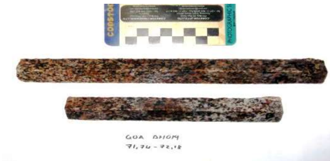
Figure 3.57 Typical Goanikontes (Etango) E-type core sample, DH019 71.74-72.18. There are distinctly oxidised portions (brick-red and black) and relatively unaltered portions in this sample (black and white colour).
