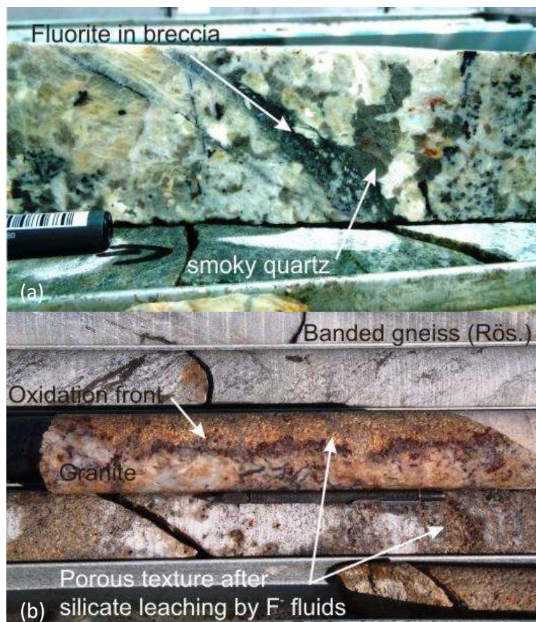
Figure 4.44 Fluorite and F-associated alteration. (a) Fluorine was mobile at some point after/during uraniferous sheeted leucogranite crystallisation. In this example a brittle fracture has cross-cut a uraniferous granite (see smoky quartz); whereas in (b) A coarse-grained pegmatoidal alaskite is less affected than its host rock, a banded gneiss of the Rössing Formation. The acidic fluid has attacked the granite leaving a front stained by mobile iron.
