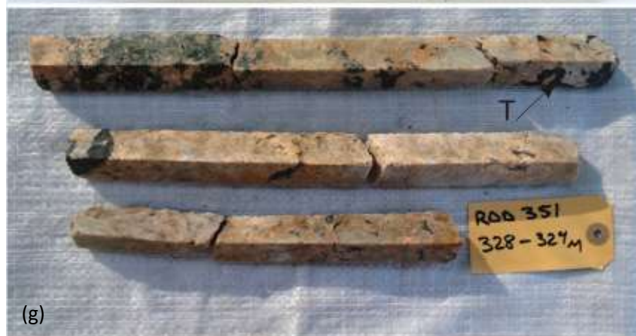
Figure 3.53 (e) and (f) Coarse-grained leucogranite with minor accessory biotite, intruded by a high - grade uraniferous quartz - biotite vein; and a granitic vein sandwiched between a banded quartzite and a quartz pegmatite (alaskite). (g) Pegmatitic sheeted leucogranite with accessory tourmaline and entrained chlorite - diopside clusters.
