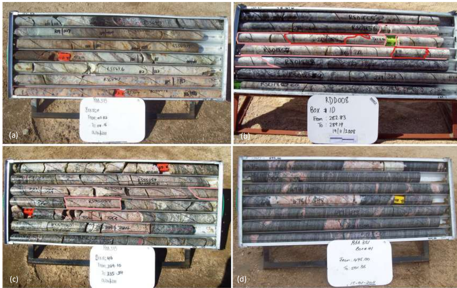
Figure 3.53 Examples of common sheeted leucogranites of the Husab Deposits. (a) An example of typical, pegmatitic textured sheeted leucogranite pegmatite that intrudes a quartzite - calcsilicate package. (b) An example of an early sheeted leucogranite, invaded by quartz - rich uraniferous granitoid. The quartz in the barren granite is distinctively milky and light coloured compared to the dark grey - black smoky quartz of the younger intrusive. (c) Magnetite - bearing leucogranite - pegmatite intruding at a low angle to bedding in Khan Formation diopside gneiss; subsequent hydrothermal fluids have altered the more porous host rocks, but much less so in the granite sheets. (d) Magnetite - bearing granite veins with characteristic pink and white feldspars and magnetite porphyroblasts. The host rock is banded diopside gneiss, Khan Formation
