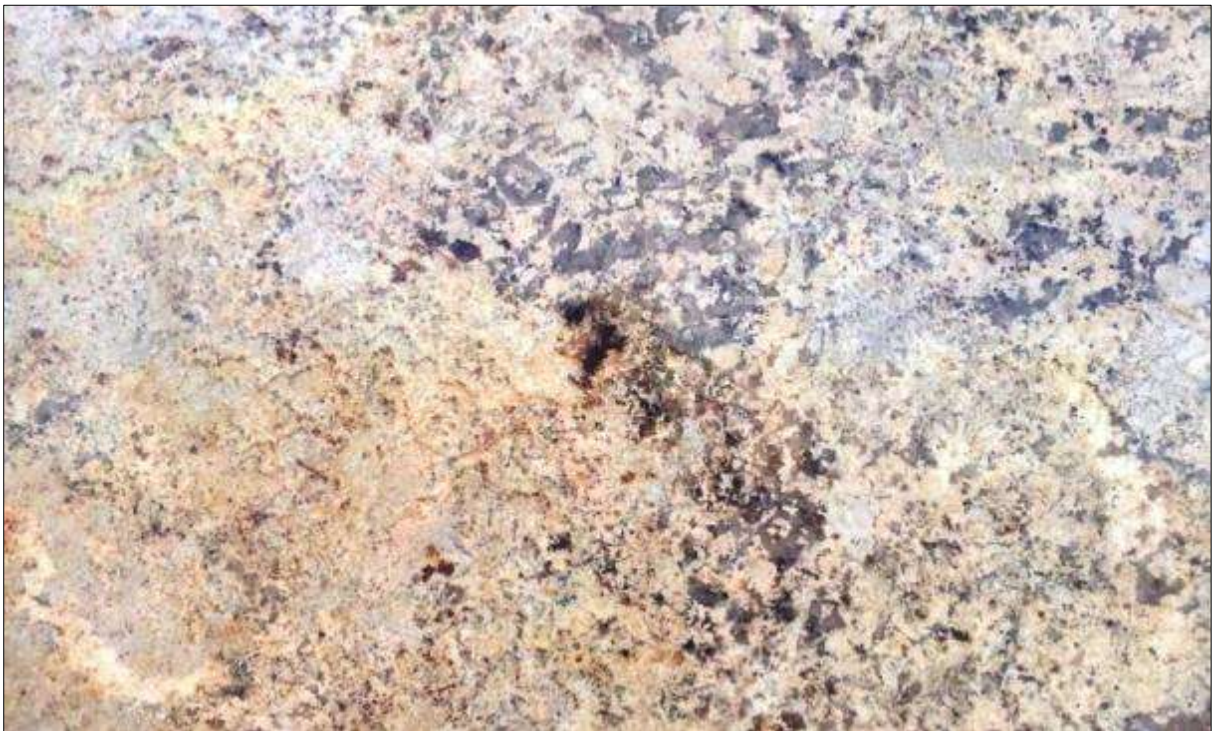
Figure 2.3 Polished slab of alaskite from the Stone Africa Quarry, SE of the Rössing Mine. Frequent local examples show more homogeneous, but coarse-grained textures that characterise most occurrences of mineralisation. Quartz is smoky as a result of radioactive disruptions to the quartz. Quartz coloration ranges from light grey (as above) to jet black, and is usually a fair indication of the U content. Field of view is approximately 50 cm.
