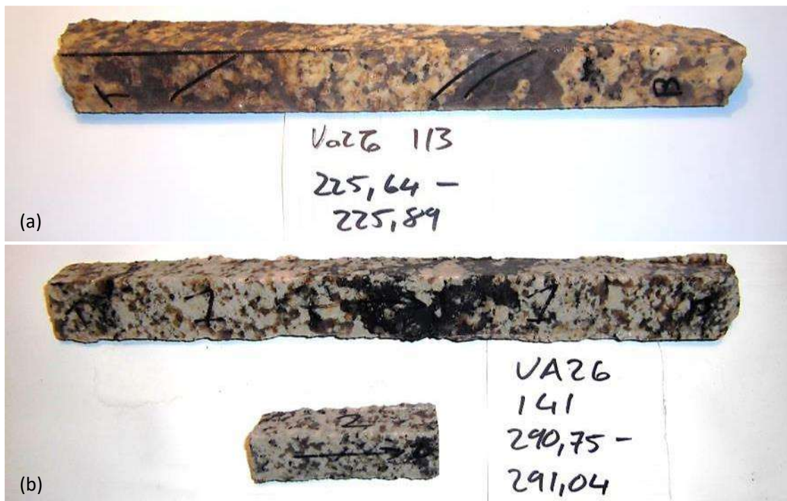
Figure 8.12 Core samples from Va26 113 and Va26 141 NQ drill holes at Valencia. (a) The 225 m interval in hole 113 is dominated by a secondary Fe overprint, analogous to the typical E-type described at Goanikontes by Nex (1997). Quartz veining and cloudy-textured feldspars are indicative of high temperature metasomatism. (b) The 290 m interval in hole 141 contains a typical Valencia sheeted leucogranite, with smoky quartz and accessory biotite indicating uranium mineralisation. Alteration is present but far less intense than in the Va26 113 sample.
