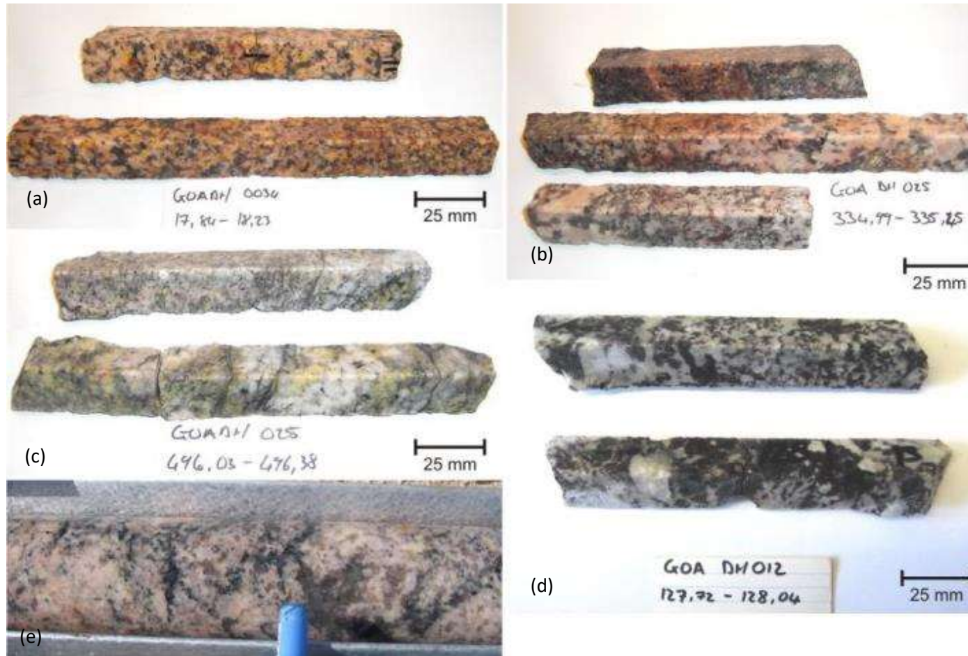
Figure 3.56 The common varieties of uranium-bearing granites observed in core from the Goanikontes Deposit. (a) Medium to coarse, homogeneous, limonite and haematite stained E-type sheeted leucogranite with accessory magnetite, alteration is attributed hydrothermal fluids. Being a shallow sample, there is likely to have been a later meteoric component. (b) Typical E-type of Nex (1997) with prominent haematite and limonite staining adjacent to unaltered granite, alteration is hydrothermal. (c) Altered sheeted leucogranite, showing sericitisation of feldspars, minor magnetite, chlorite streaks and veins, with biotite, inhomogeneous texture and brecciation, potential for alteration fluid migration along fault pathways. (d) Typical D-type of Nex (1997) with variable coarse texture, jet black smoky quartz and white feldspars. (e) Significant reaction with surrounding
