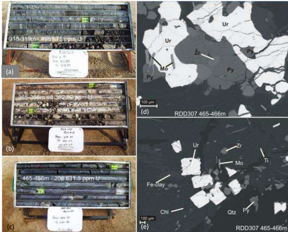
Figure 4.40 Pegmatitic uraniferous sheeted leucogranites at the Husab Deposit, Zone 1. (a) Coarse-grained biotite books, occupy 20 to 30 cm spaces within the pegmatite and host the majority of the U. The intrusion is ~5 m thick and intrudes mottle-textured cordierite gneiss of the Rössing Formation in drill hole RDD023. (b) Similarly, a centimetric - scale patch of very coarse biotite books hosts significant U in a 29-m thick interval of uraniferous sheeted leucogranite. The biotite clusters occur within 80 cm of the footwall contact with intercalated gneiss and calcsilicate of the Rössing Formation, RDD078. (c) The highest-grade sample from Husab occurs in Zone 1 and comprises almost entirely biotite with subordinate quartz. The biotite is entirely chloritised, with interstitial spaces between books and clusters filled by smoky quartz, RDD307. (d) and (e) Backscatter images of the RDD307 465 m interval: The host phase is almost entirely uraninite which occurs in two distinct textures. The primary uraninite is euhedral and cubic, 100 µm to 500 µm across and assembled in clusters with sulphides between biotite (chloritised) books. The secondary texture fills spaces between the gangue phases and contains inclusions of earlier - crystallised minerals (pyrite in Figure d).
