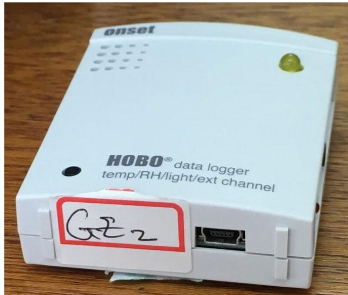
Figure 3.4: Onset HOBO U12-012 Temp/RH/Light/Ex sensor
