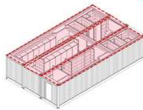
Steel Structural Frame 9 meters x 8.5 meters
