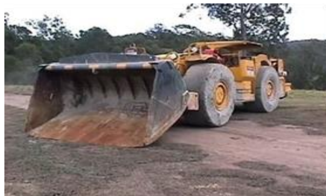
Figure 2.5: Load Haul and Dump (LHD) vehicles
