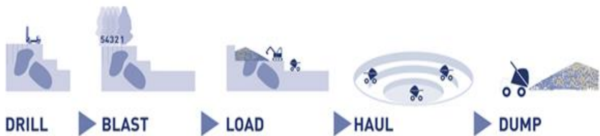
Figure 2.2: The cycle in opencast mining
