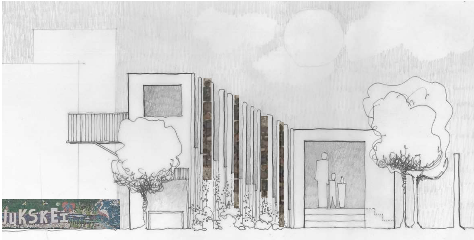
Figure 2.20: Elevation of the tower with the observation deck cantilevering out over the river
