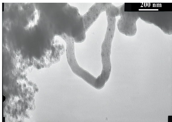
Figure 7.4: TEM image of CFs formed at 900 °C, ( \text{CpFe(CO)}_2\text{Me} : 5 wt.%; 0.8 ml/min injection rate)
