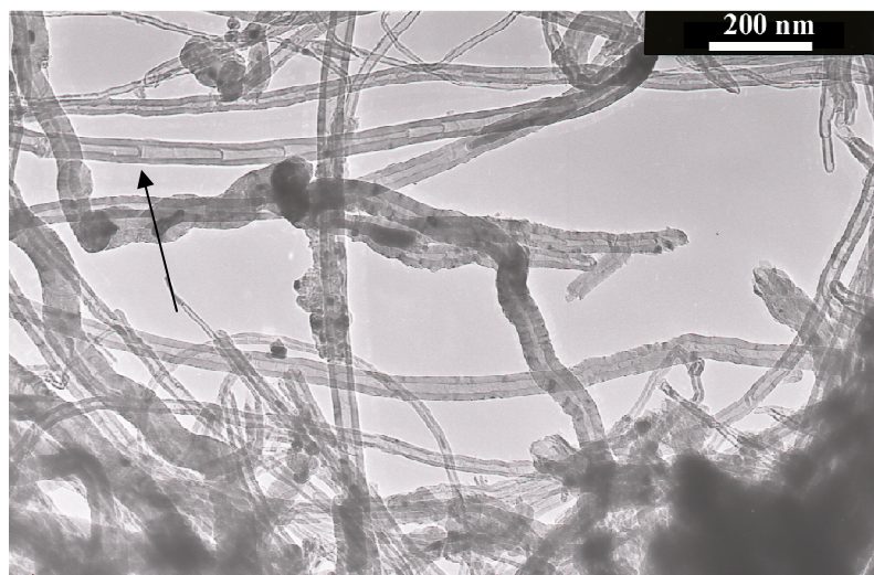
Figure 6.1: TEM image of N-doped MWCNTs formed using diisopropylamide catalyst (800 °C, 0.8 ml/min 2.0 wt%) ( arrow = bamboo structure )
