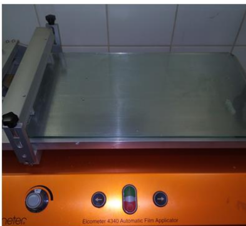
Fig. 1. Casting machine for PIM preparation
