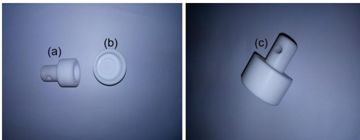
Fig. 3. A representation of receiving chamber for a solution (a), screw cap showing a window opening where the membrane is placed (b) as well as closed passive sampler device (c).
