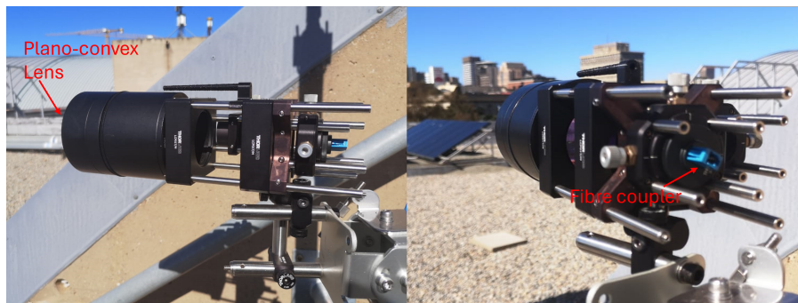
Figure 5.8: Experimental bidirectional FSO system. The system utilises a plano-convex lens with a diameter of 75 mm and focal length of 200 mm.
