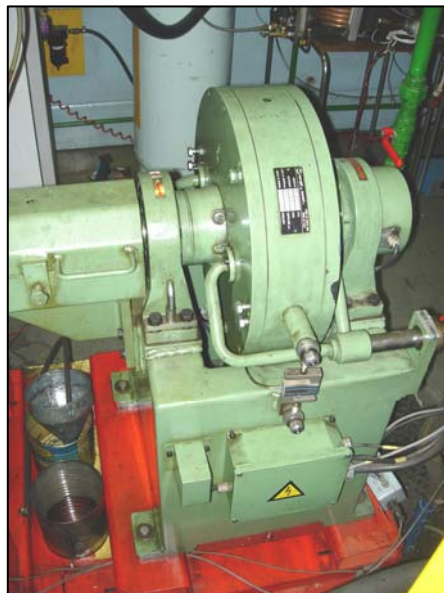
Figure 5-3: Borghi & Saveri Dynamometer
