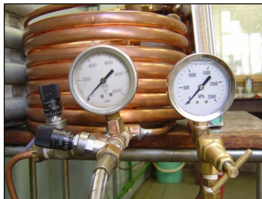
Figure 5-11: Prototype helical heat exchanger
