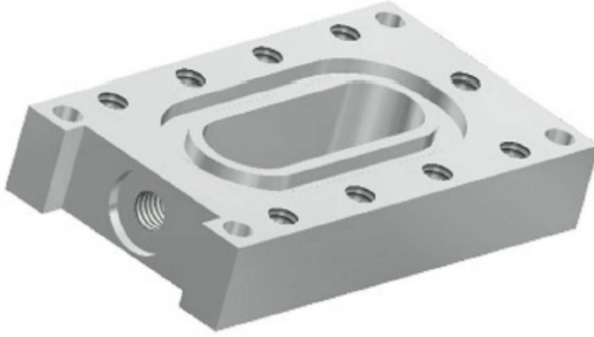
Figure 3.4: A drawing of 10 mm thick gas target cell.
