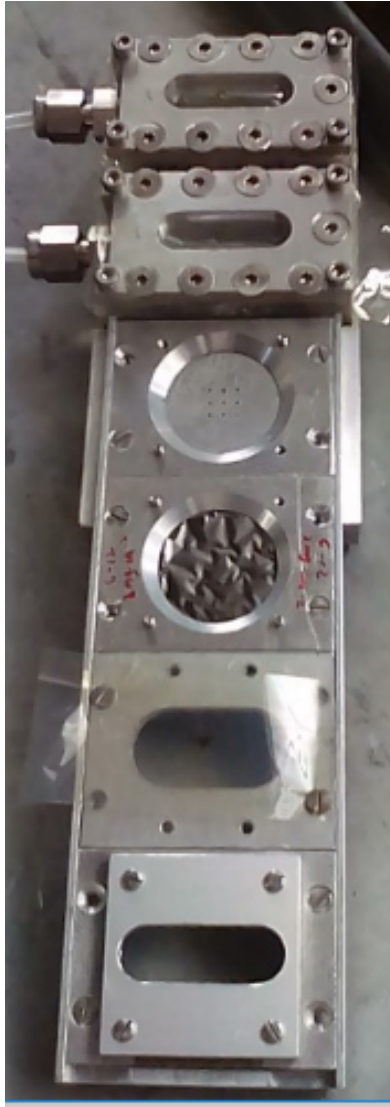
Figure 3.5: The target ladder with two gas cells at the top.
