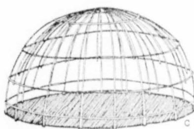
a. Sotho beehive hut framework: after Walton. b. Zulu/Swazi beehive hut framework. c. Xhosa beehive hut framework: after Walton.
