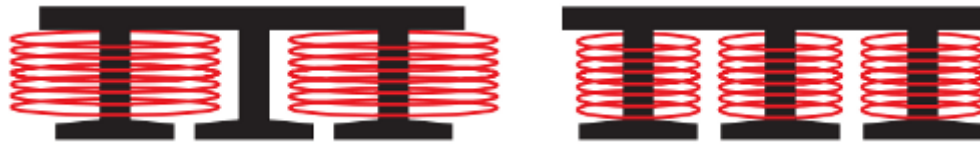
Figure 33: Single versus double layered windings [48]
