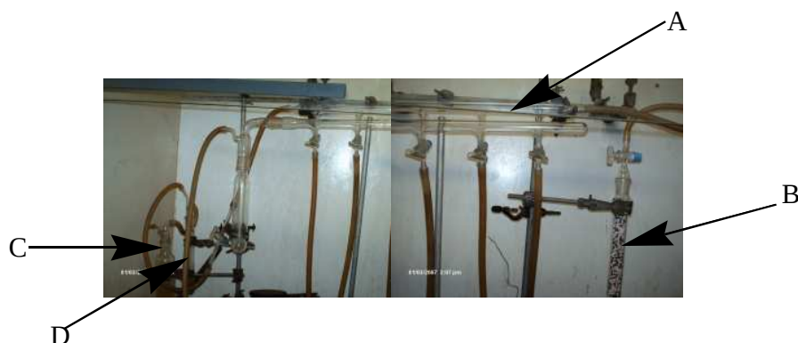
Figure 3.1. Manifold nitrogen line
