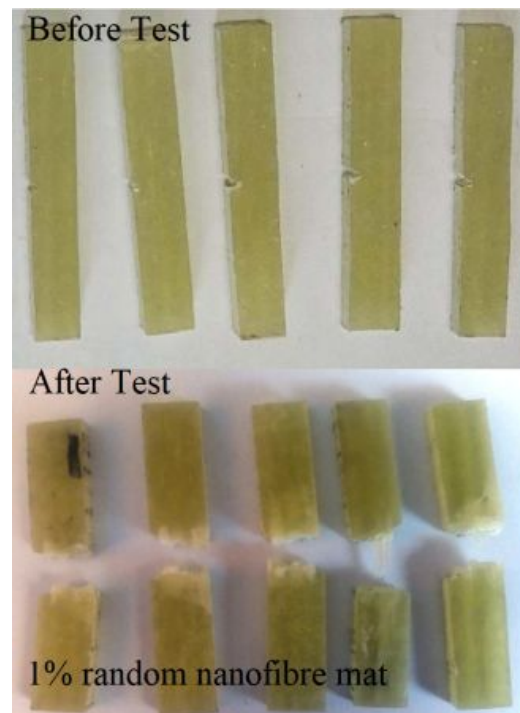
FIGURE A.37: Tested impact specimens of Random nanofibres mat (1% Vol) strengthened hybrid composite
