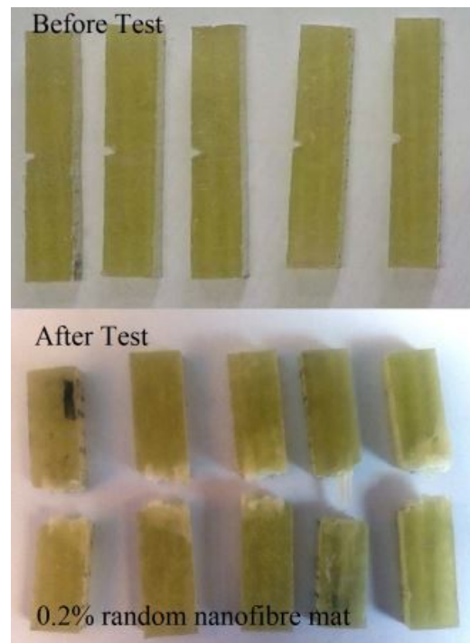
FIGURE A.35: Tested impact specimens of random nanofibres mat (0.2% Vol) strengthened hybrid composite
