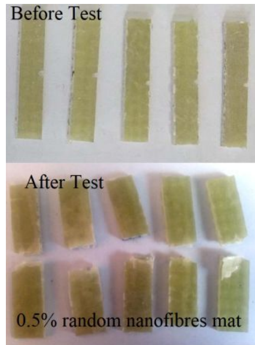
FIGURE A.36: Tested impact specimens of Random nanofibres mat (0.5% Vol) strengthened hybrid composite
