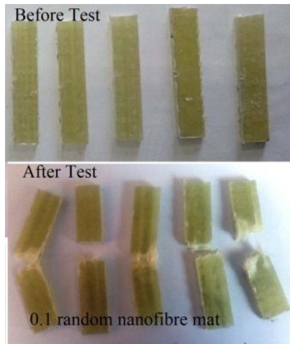
FIGURE A.34: Tested specimens of Random nanofibres mat (0.1% Vol) strengthened hybrid composite samples
