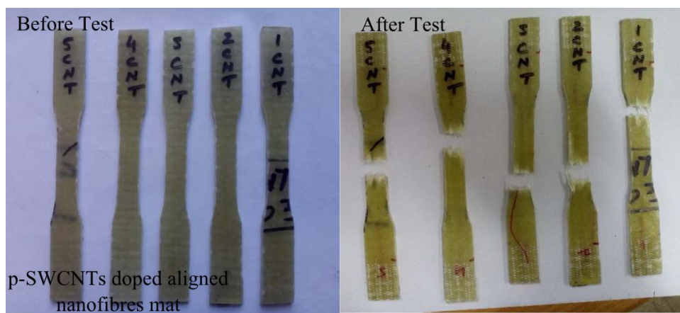
FIGURE A.14: Tested Tensile specimens of p-SWCNTs (vol 0.25%) doped aligned nanofibres mat (0.5% vol) strengthened hybrid composite samples
