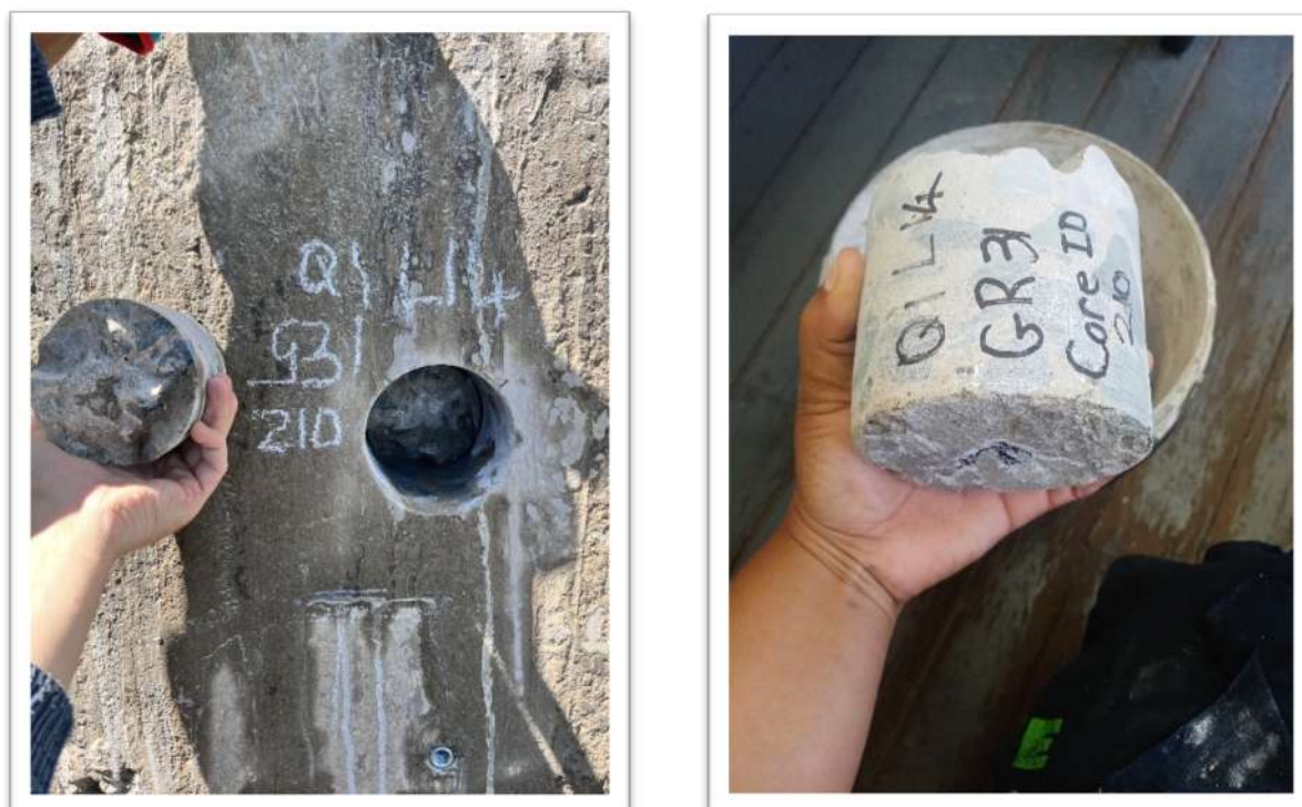
Figure 0-4 Core extracted from Quarter 1 level 14
