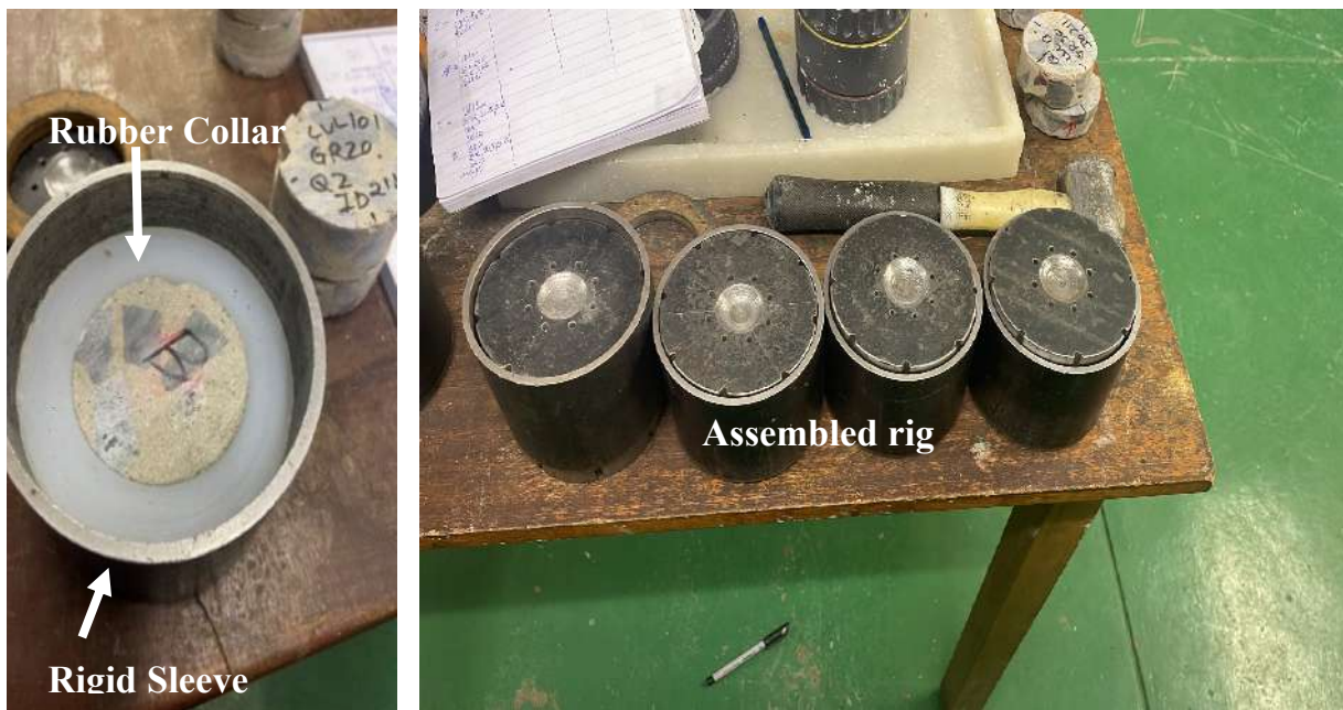
Figure 3-17 – Samples being inserted into the collar.
