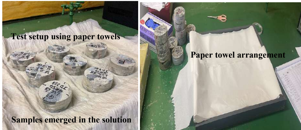
Figure 3-12: Water Sorptivity Test being carried out in the laboratory.
