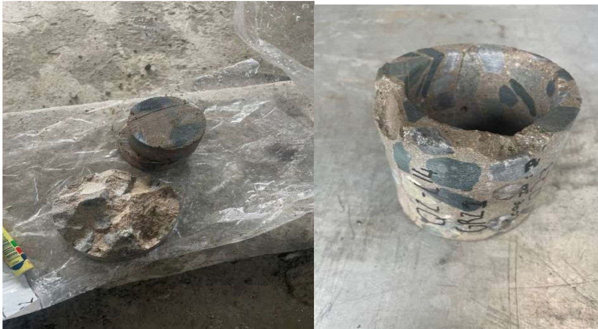
Figure 3-9: 70mm durability specimen extracted from a 100mm core.
