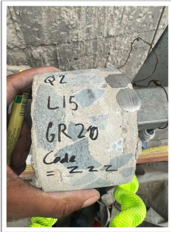
Figure 0-5 Cores extracted from Quarter 2 level 15
