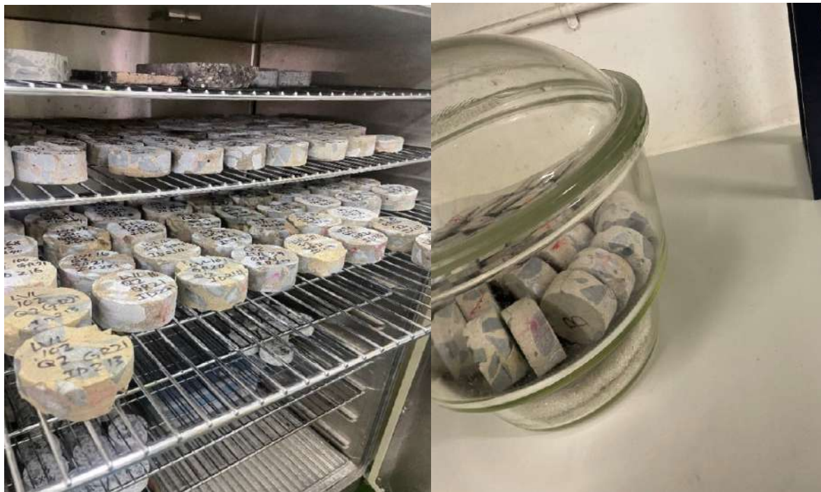
Figure 3-10: Durability specimens discs being dried in the oven and dessicator.
