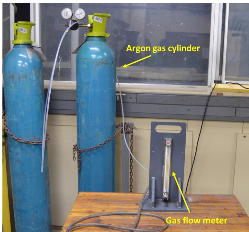
Figure A16: Argon gas cylinders and a Fischer & Porter Model 10A6132M/B10 - 1/4" NPTF gas flow meter.
