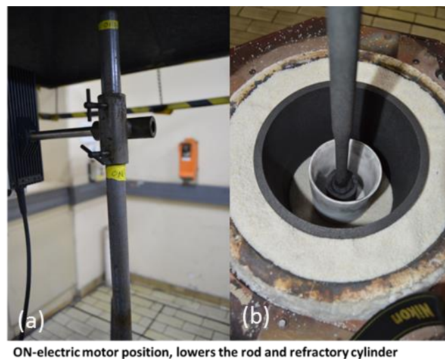
Figure A10: Marked position for the rotating motor (a) and the refractory cylinder level when lowered to 'On' position (b)
