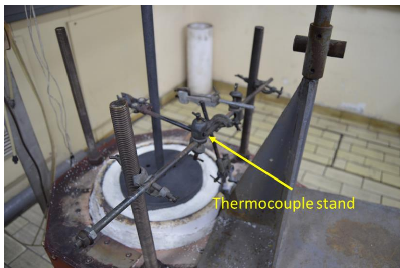
Figure A13: Thermocouple stand used for mounting tubes
