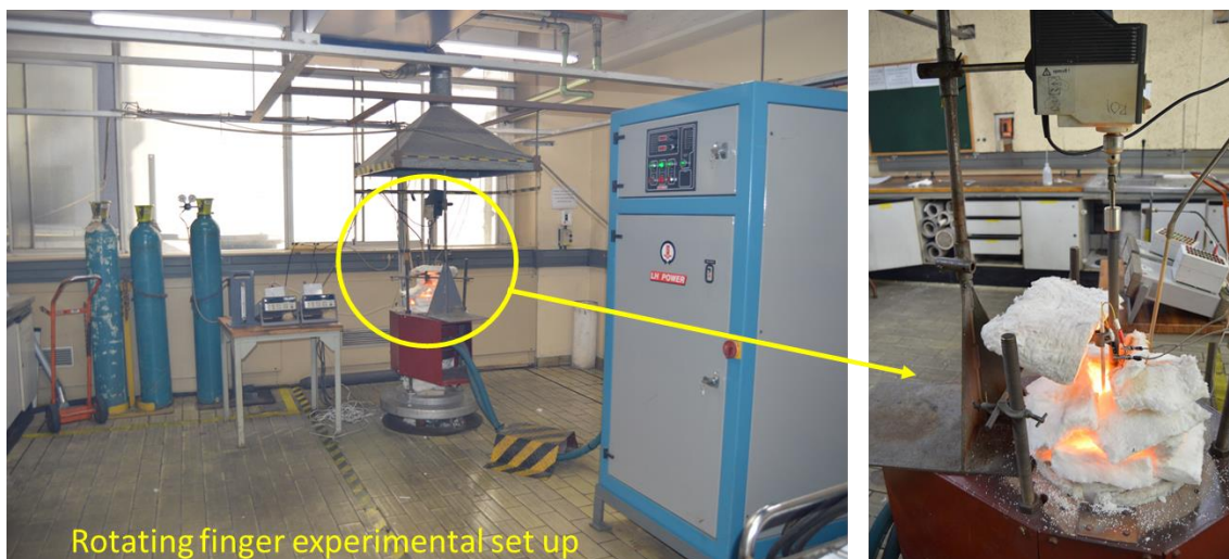
Figure A22: Complete rotating finger experiment (left) and closer view (right)
