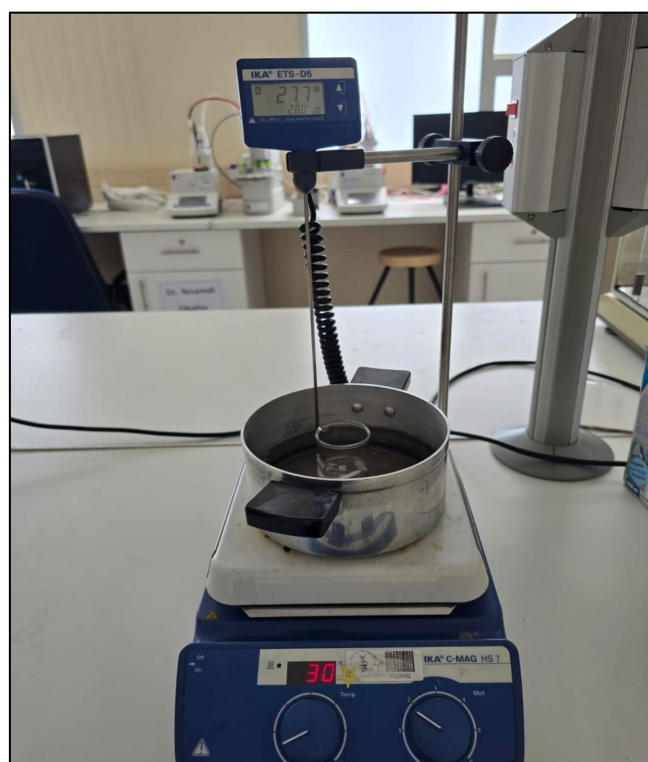
Figure 5.2. Representation of the magnetic stirrer assembly used for the stirring magnetic bar method.
