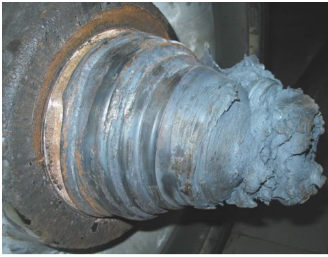
Figure 4. Rail axle failure due to over-heating of the roller bearing. 41,72
