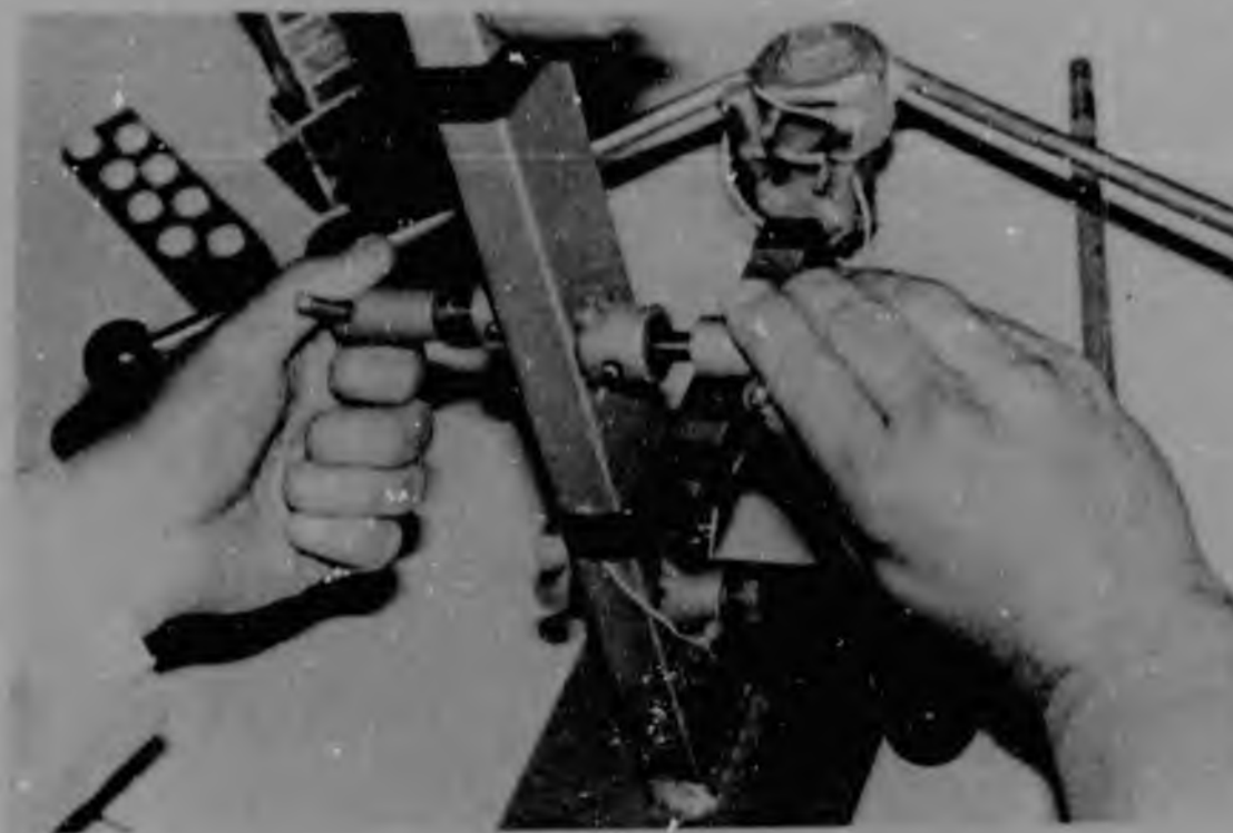
Figure 41 Test 9 showing hands tightening tap handles simultaneously
