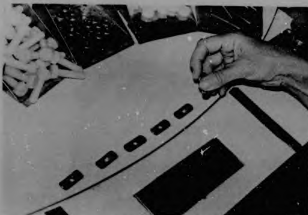
Figure 90 Test 53 showing the plate being turned through 180 degrees using the fingers
