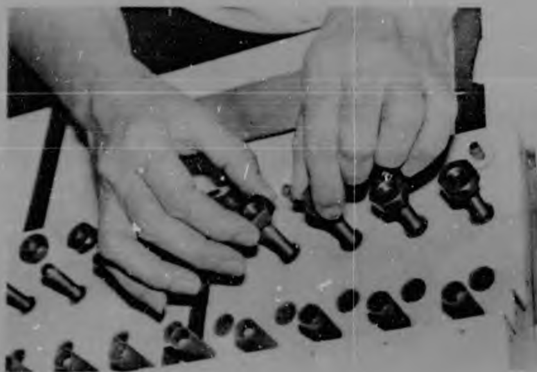
Figure 31 Test 41 shows both hands positioning the second of five nuts on bolts held in jigs. Note that the bolts are in the jigs nearest the testee.
