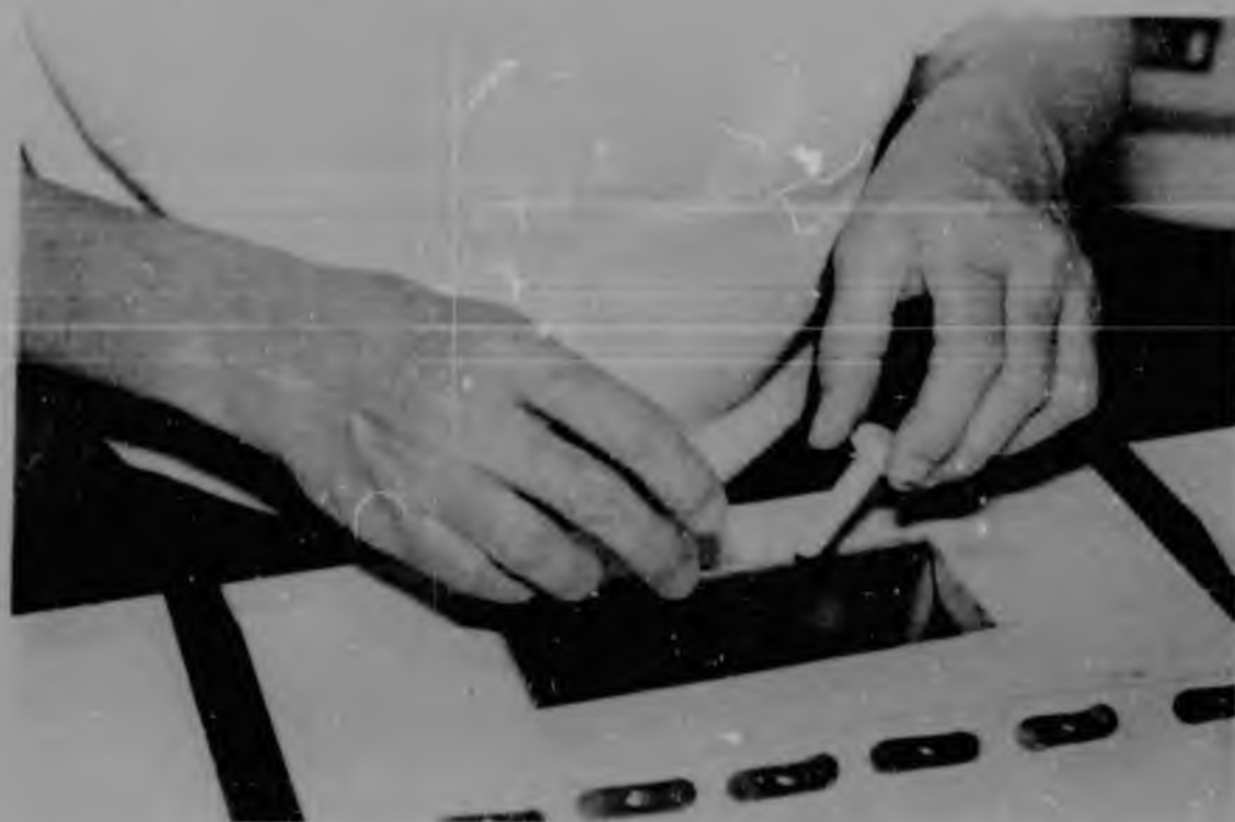
Figure 94 Test 28 showing the nut and bolt being dropped unassembled down the chute
