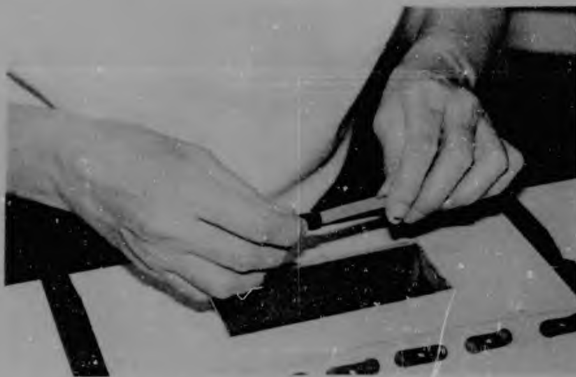
Figure 93 Test 31 showing the pen and pen top being assembled before being dropped down the chute
