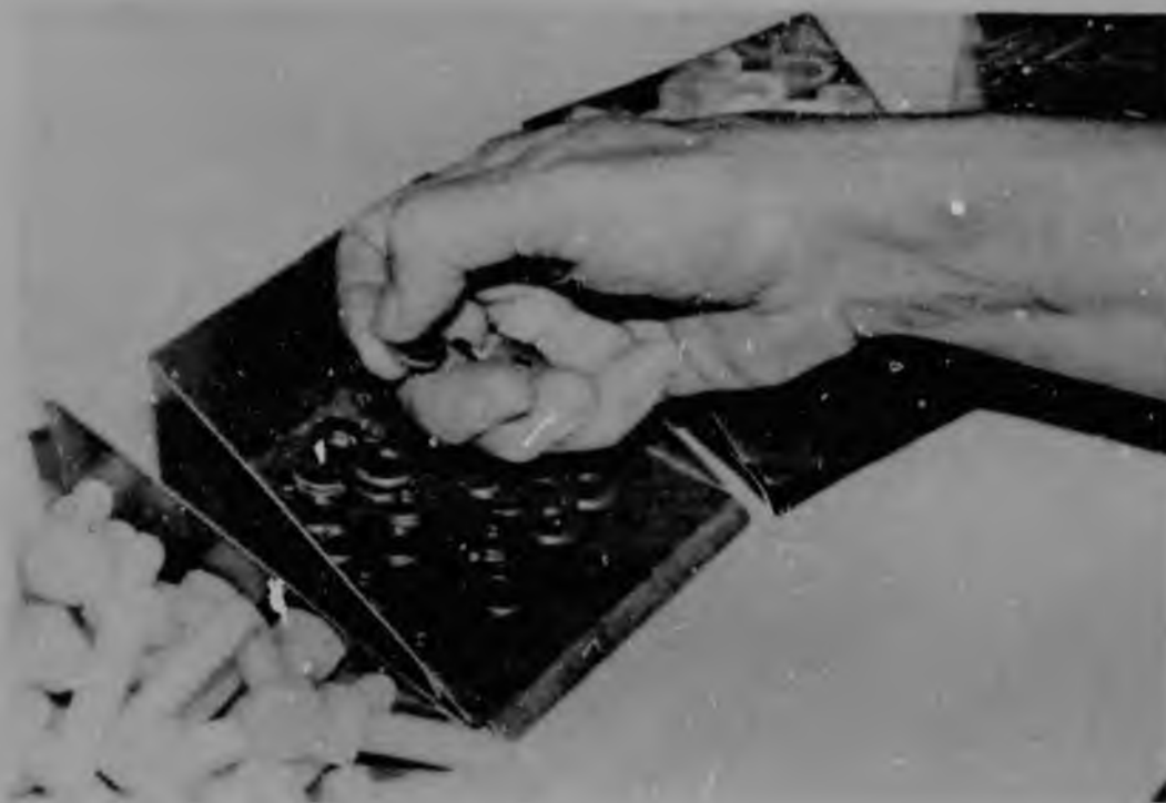
Figure 89 Test 54 showing a washer being palmed with others after being picked up from the bin
