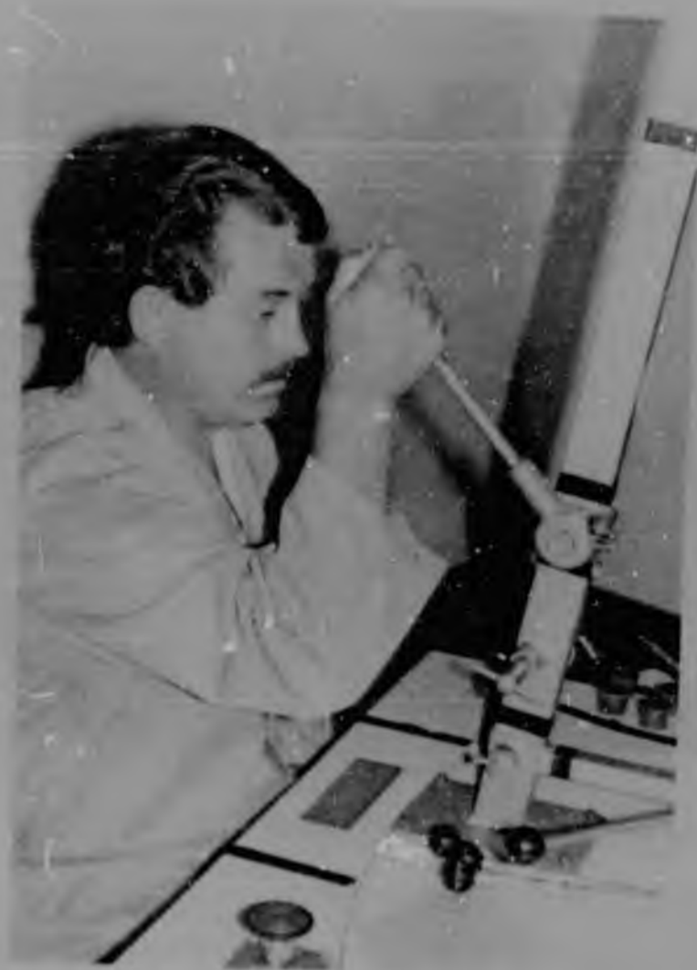
Figure 46 Test 44 showing handle C being pulled downwards, while the testee is seated
