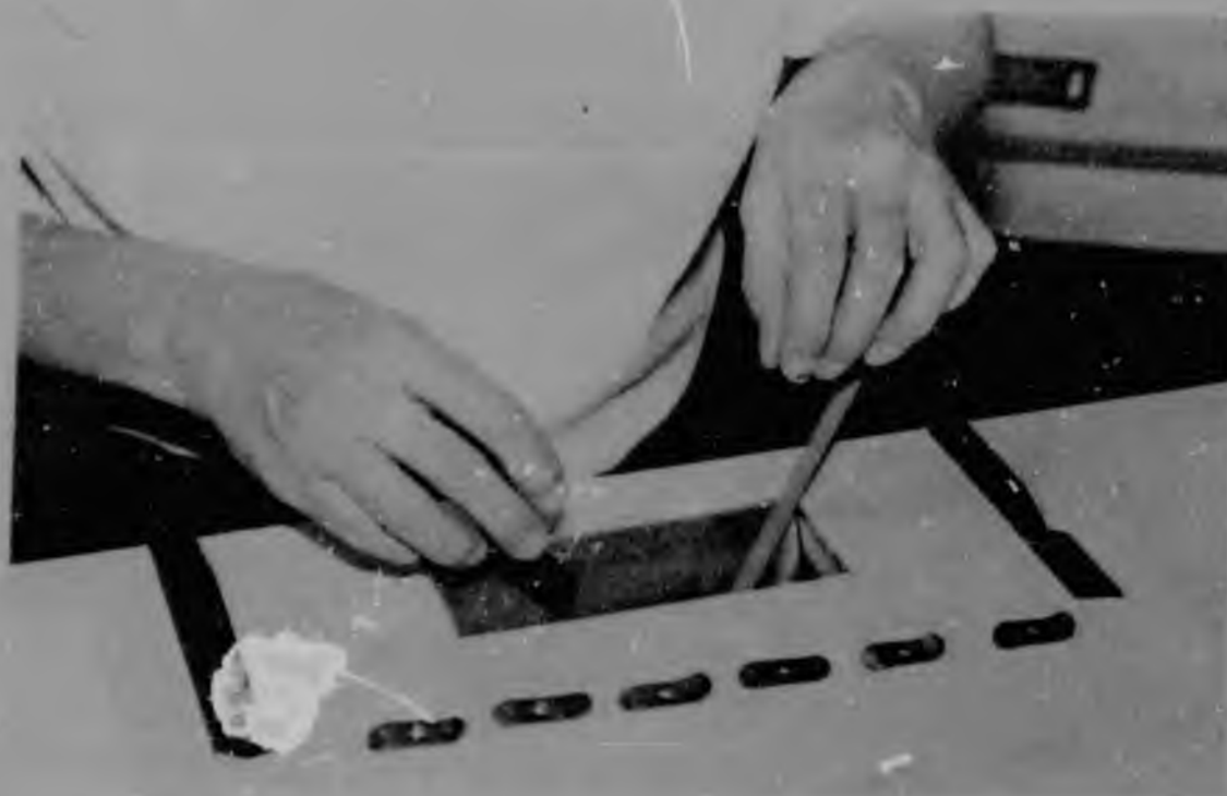
Figure 92 Test 29 showing the pen and pen top being dropped unassembled down the chute
