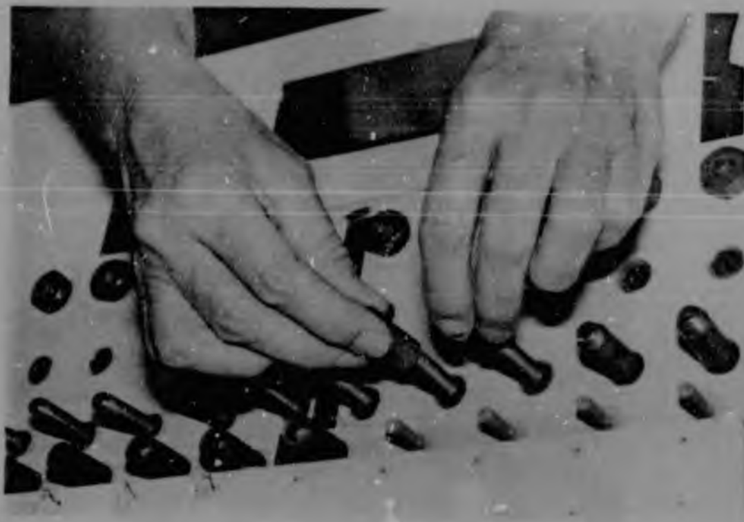
Figure 33 Test 32 showing two bushes being placed over two adjacent bolts
