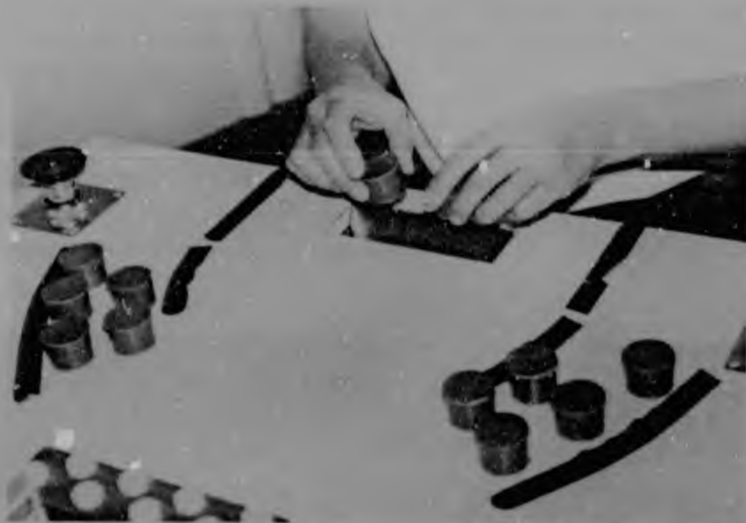
Figure 21 The width of the chute mouth accommodated bi-lateral disposal of components. BMW table.
