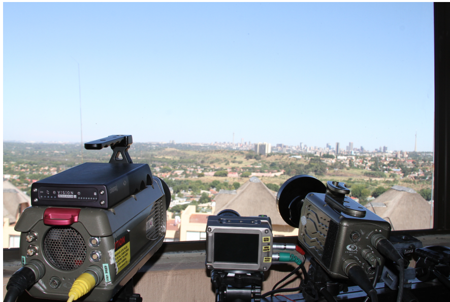
FIGURE 3.5: The set-up of the Phantom v310 (far left) and the Phantom v7.1 (far right) high-speed cameras.
