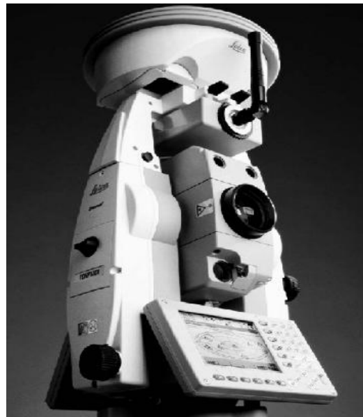
Figure 2.3: The combination of Total Station and GPS – Smart Station (Source: Hill, 2005)
