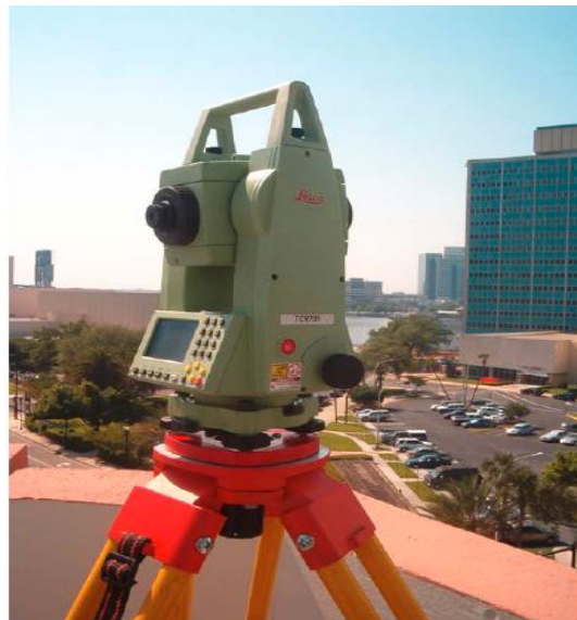
Figure 2.2: Leica TCR 705 Reflectorless Total Station (Source: Leica Geosystems online product site).
