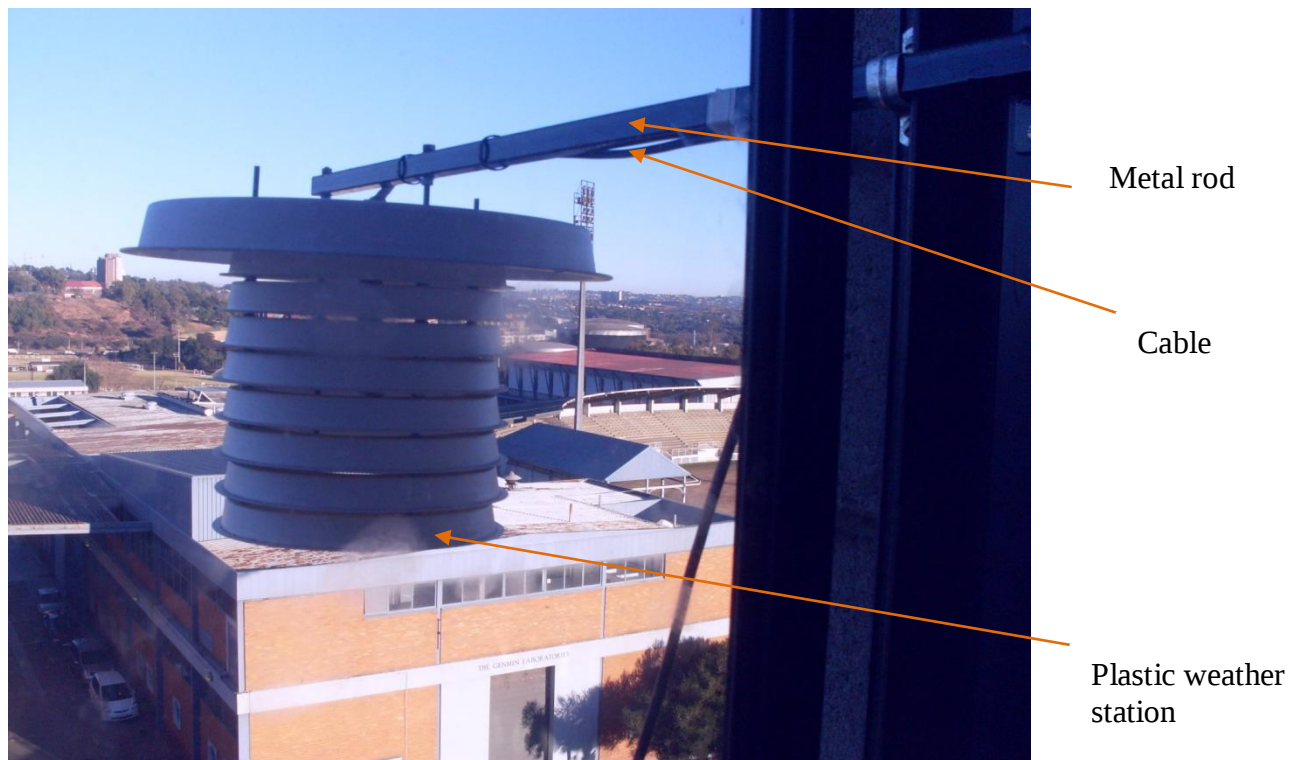
Figure 4.11: Weather station and the DTM Meteo sensor
