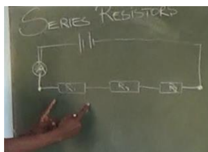
Photograph 55(b) Resistor connected in a series
