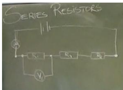
Photograph 56(a): Voltage across series resistors
