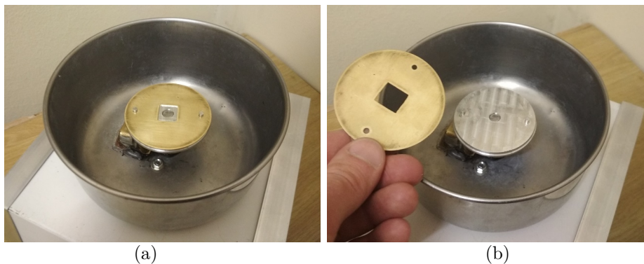
Figure 4: Final sample chuck design used for hV2 employed smooth pins machined out of the same block of aluminium as the chuck itself. (a) Chuck with the sample mask and a glass substrate in place, (b) Chuck with the sample mask removed.
