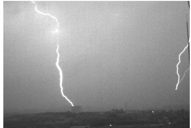
Figure 11. Downward bipolar flash struck the building and triggered an upward leader from a 250 meter-tower 2 kilometer away.
