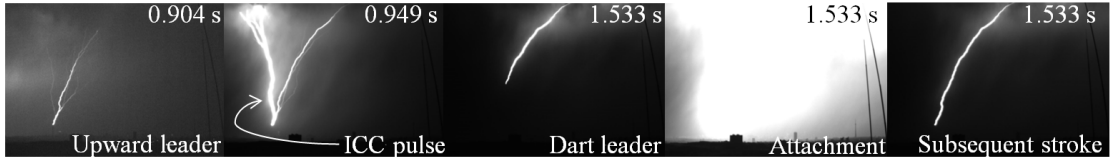
FIGURE 3.5: The different processes in upward flashes caught with a high-speed camera
