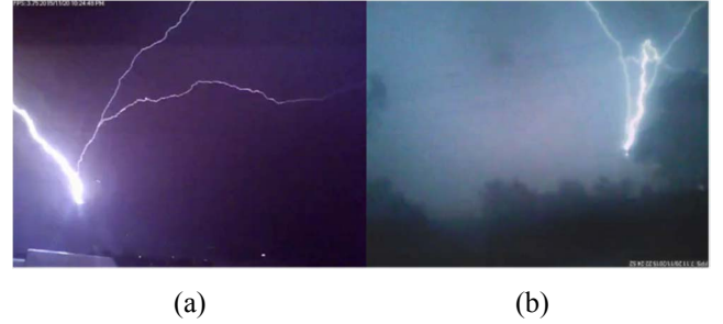
Figure 6. A lightning strike to the Brixton tower on the 20 November 2015 at 22:24:48 SAST. Two cameras observe the Brixton tower – (a) one situated at WITS university and facing east, (b) the other situated 1 km north of the tower and facing south.
