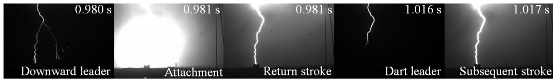
FIGURE 3.4: The different processes in downward flashes caught with a high-speed camera
