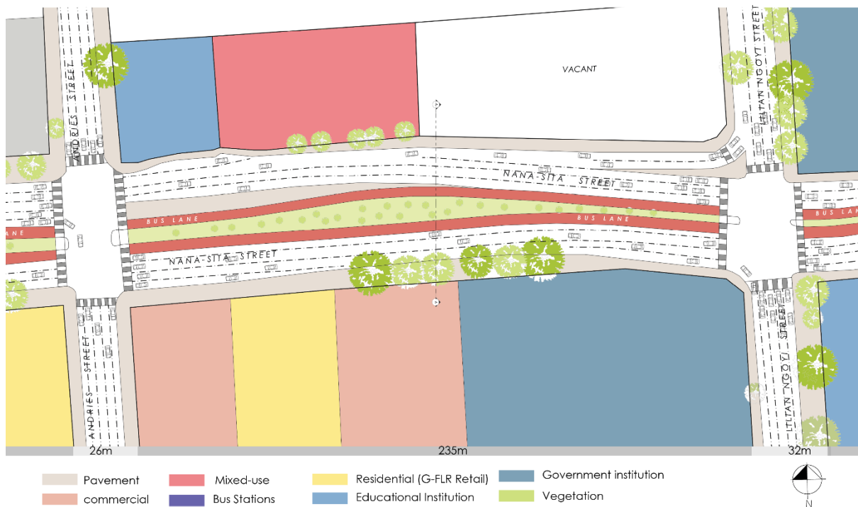
Figure 8: The map indicates street form, block size and land uses on Nana-Sita Street. (Drawn by Tswai, 2021).
