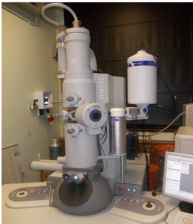
Fig. 3.4: FEI Tecnai G 2 Spirit electron microscope used to study the GaN NSs.
