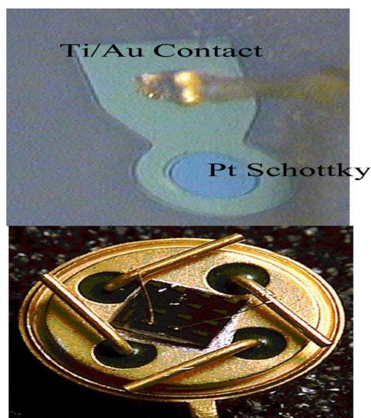
Fig. 2.26: SEM micrograph of completed device, showing bond wire attached (top) and photograph of device bonded into header [86].
