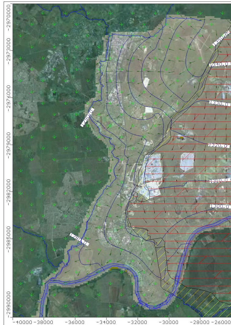
Figure 1-4: Hydrogeological model used in this study. Green symbols indicate lava, yellow cross lines indicate quartzites and the red lined area indicates dolomite. Blue lines indicate contours of equal water table level with the contours shown for the water table in mamsl. Black arrows show the direction of water flow based on head measurements in the boreholes. Coordinates are for the LO27 projection on the WGS84 datum (in metres, from De Sousa et al. , 2006).
