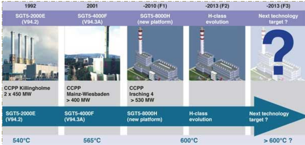
Figure 2.5: Improvements in Siemens Gas Turbine Combine Cycle (COSPP, 2014)
