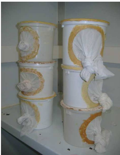
Figure 3.2 Plastic cages (2.5 l) used for fungal exposures; 3 served as controls and 3 as treatments.
