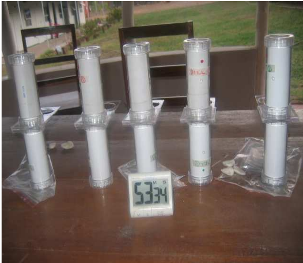
Figure 4.4 World Health Organization experimental set-up for insecticide susceptibility tests in Karonga, Malawi.
