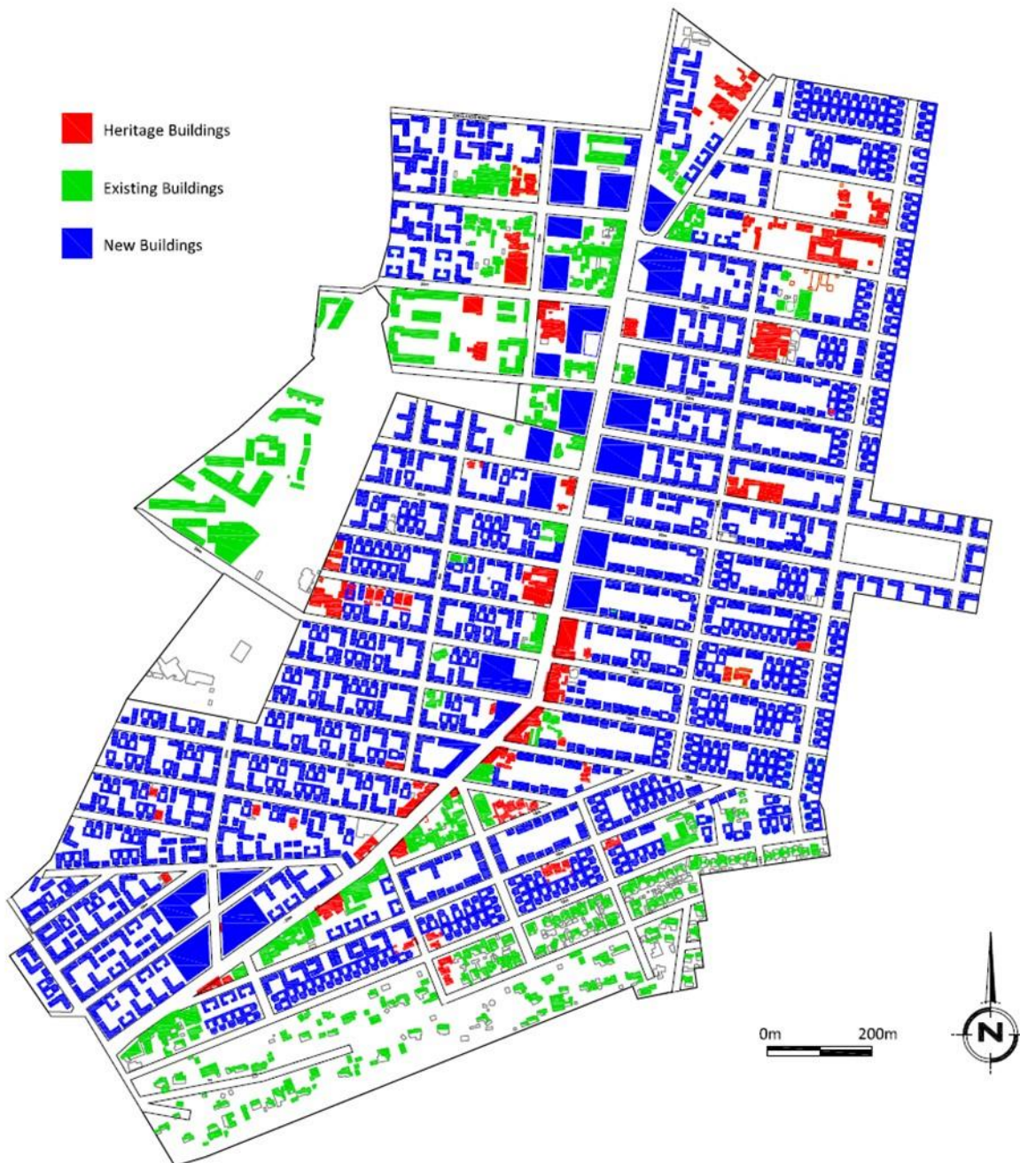
Figure 5. 14: Site Map 11 – roof space identified with potential for PV in Orange Grove (Source: based on the COF SDZ, 2017)
