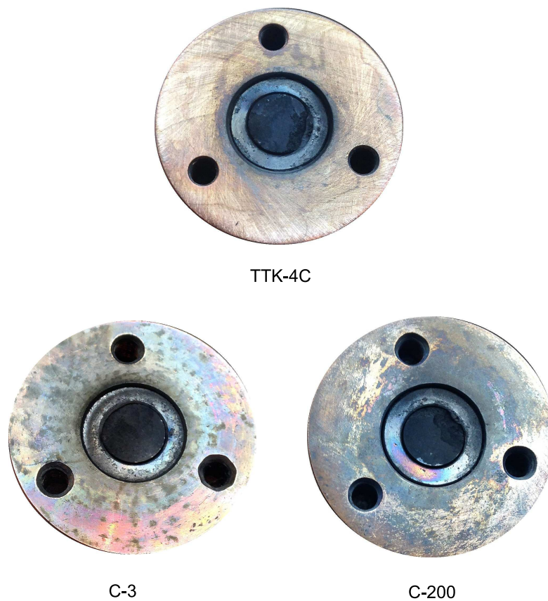
Figure 7.3: Photographs of cathode erosion for TTK-4C, C-3 and C-200 copper-impregnated carbon graphite rods.
