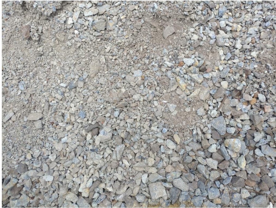
Figure 9: Gravel for constructed wetland bed media that was procured from a local supplier in Silvertown, Alexandra
