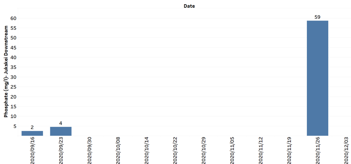
Figure 62: Results from phosphate concentration (mg/l) tests conducted on samples from the Jukskei River upstream and downstream of Alexandra
