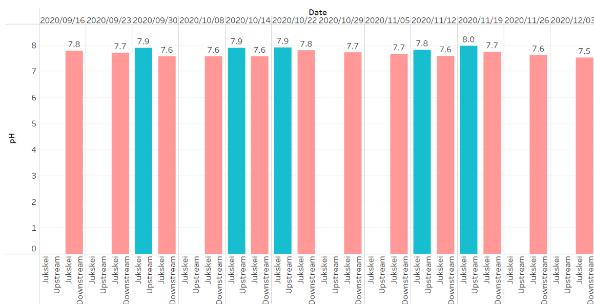
Figure 57: Results from pH tests conducted on samples from the Jukskei River upstream and downstream of Alexandra
