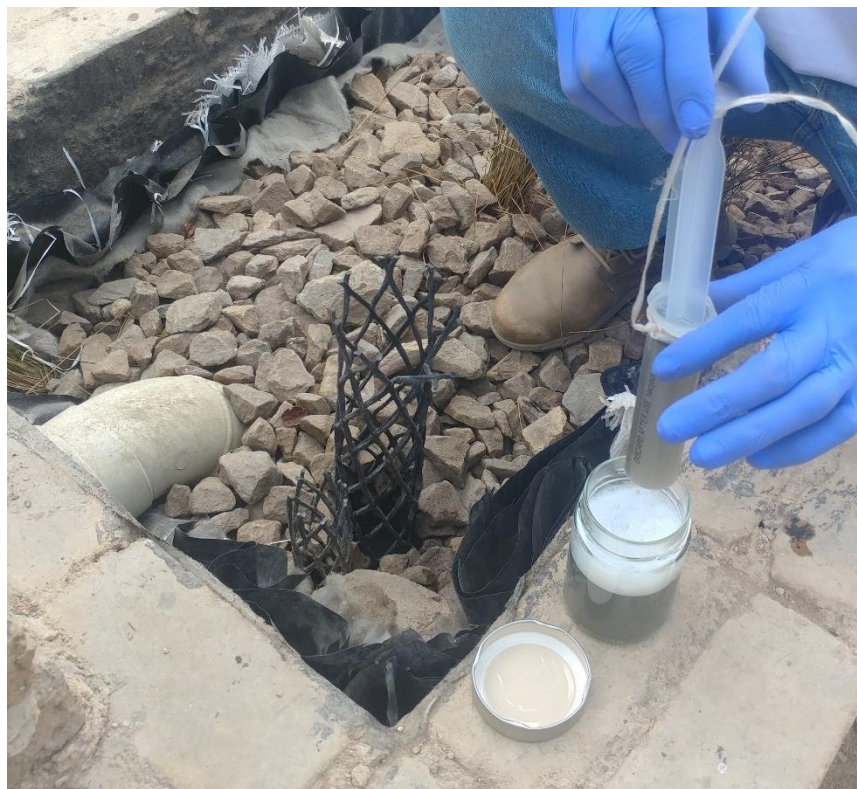
Figure 27: Syringe and glass jars used for sampling. The access point to the water beneath the gravel level is in the black mesh cylinder in the centre of the photograph.
